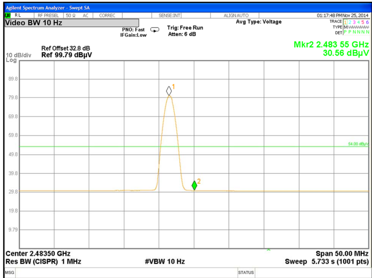
Figure 47: Radiated Emission at the Edge for Channel 2480 MHz at 1Mbps BLE mode– Horizontal (Avg)
