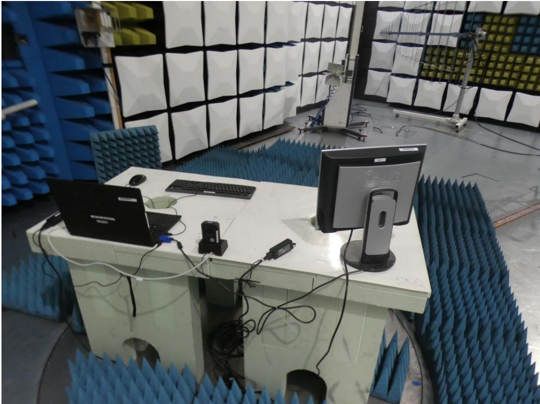
Photo 7: Test setup S03_AA01 for radiated emissions measurements above 1 GHz
