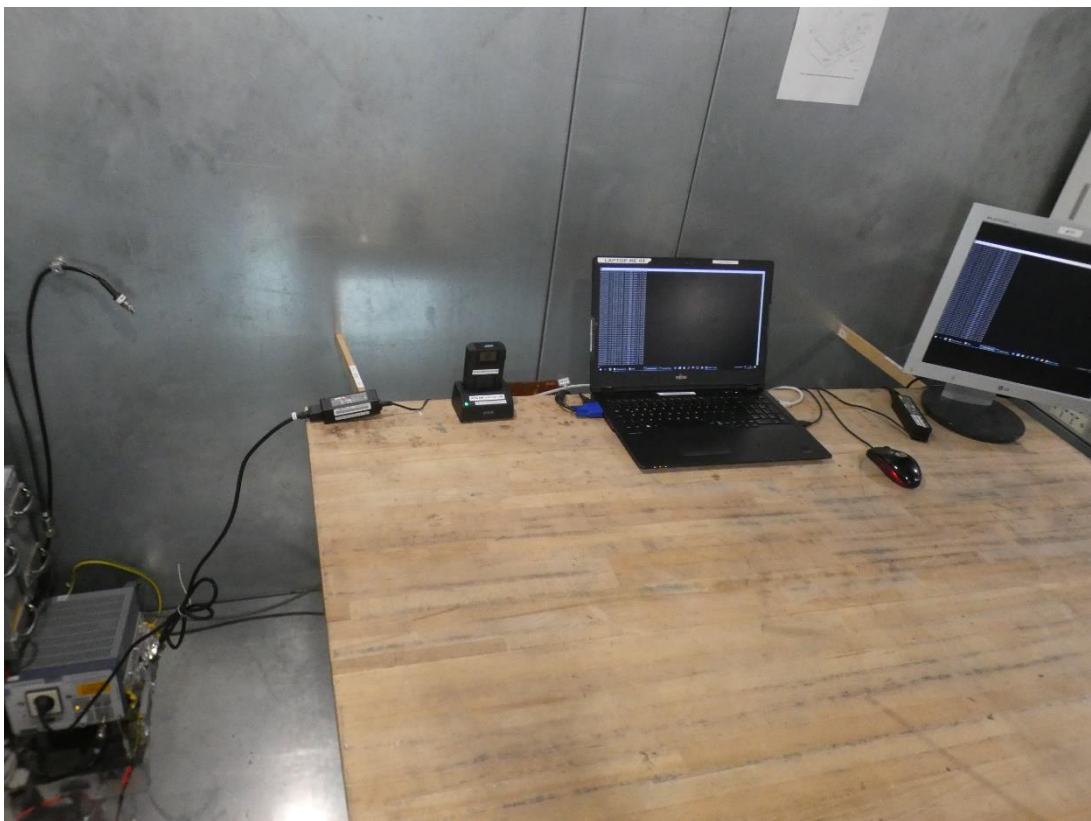
Photo 2: Test setup S03_AA01 for conducted emissions measurements below 30 MHz
