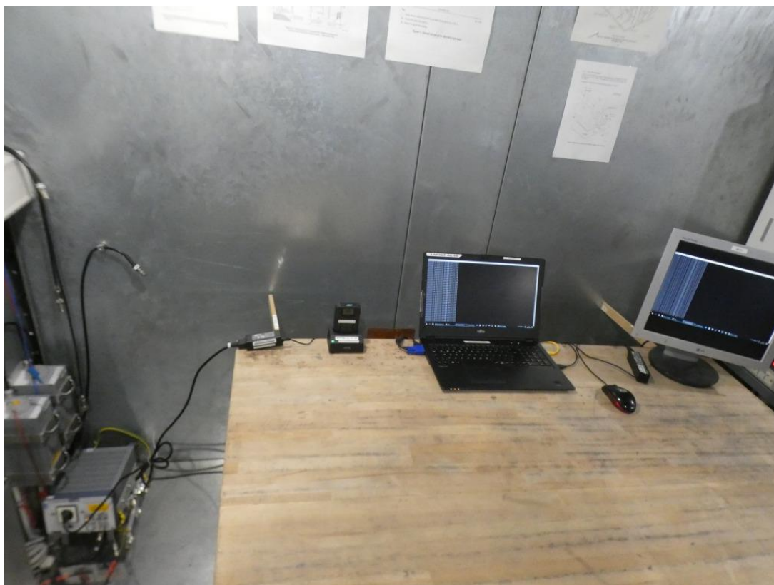
Photo 3: Test setup S04_AA01 for conducted emissions measurements below 30 MHz
