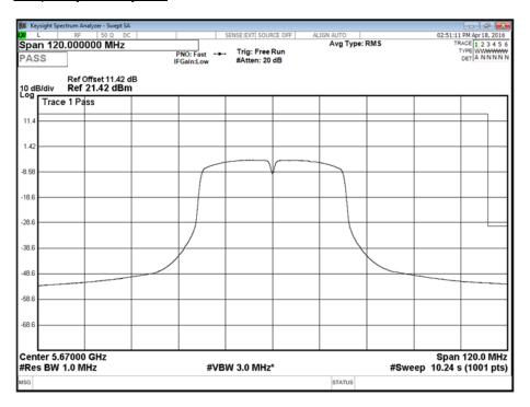
802.11n - 5 GHz 40 MHz Bandwidth, 5670 MHz, +55.0, 4.0 V DC, Frequency Band 3, Frequency Stability Plot
