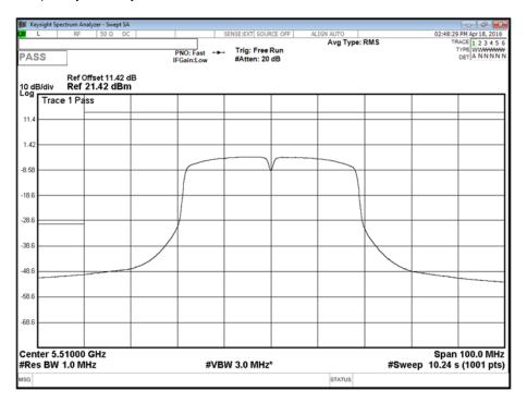
802.11n - 5 GHz 40 MHz Bandwidth, 5510 MHz, +55.0, 4.0 V DC, Frequency Band 3, Frequency Stability Plot
