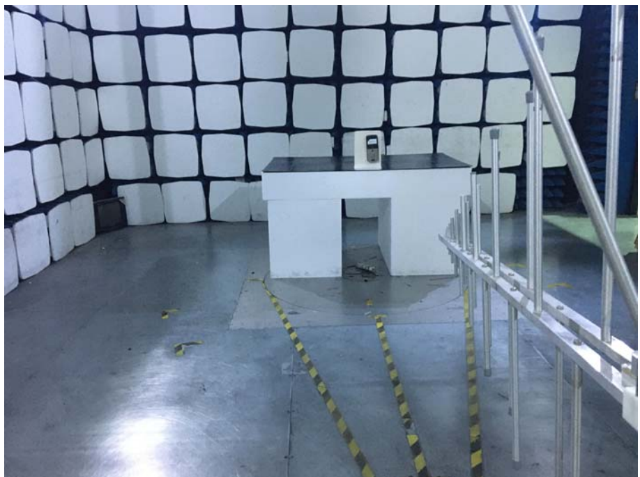
Radiation Emission Test Setup (30MHz to 1GHz)
