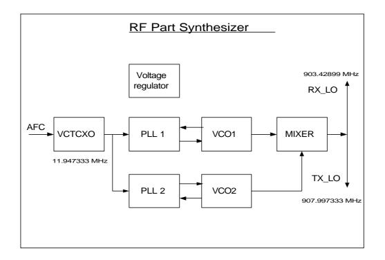
The clock sourse based on a standard VCTCXO controlled by the CPU. The compensation value is calculated and it is using to control the VCTCXO. The multiplier output is filtered by BPF to achieve the requirements of the LO.
