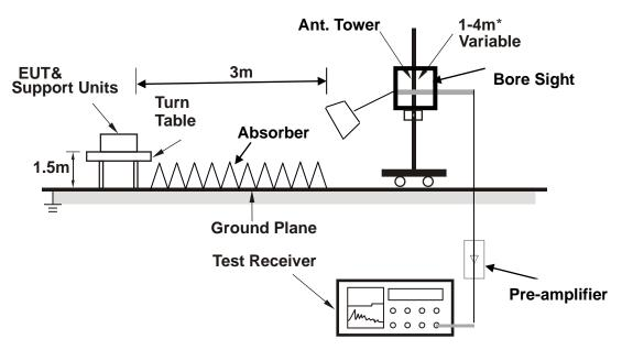
**Note**: Above 1G is a directional antenna depends on the EUT height and the antenna 3dB beamwidth both, refer to section 7.3 of CISPR 16-2-3.
