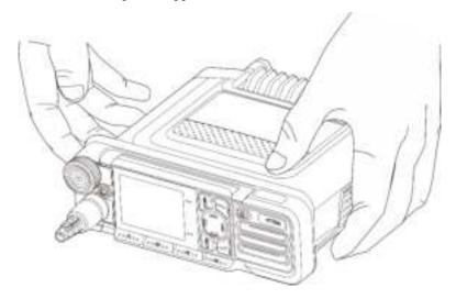
Hold the front panel, and then pull and remove the plastic upper cover.
