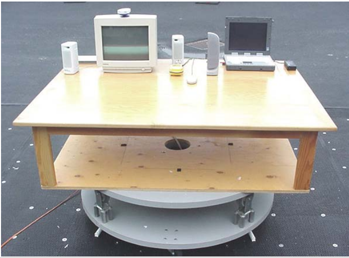
Photograph F-3 - Front of Radiated Emission Configuration
