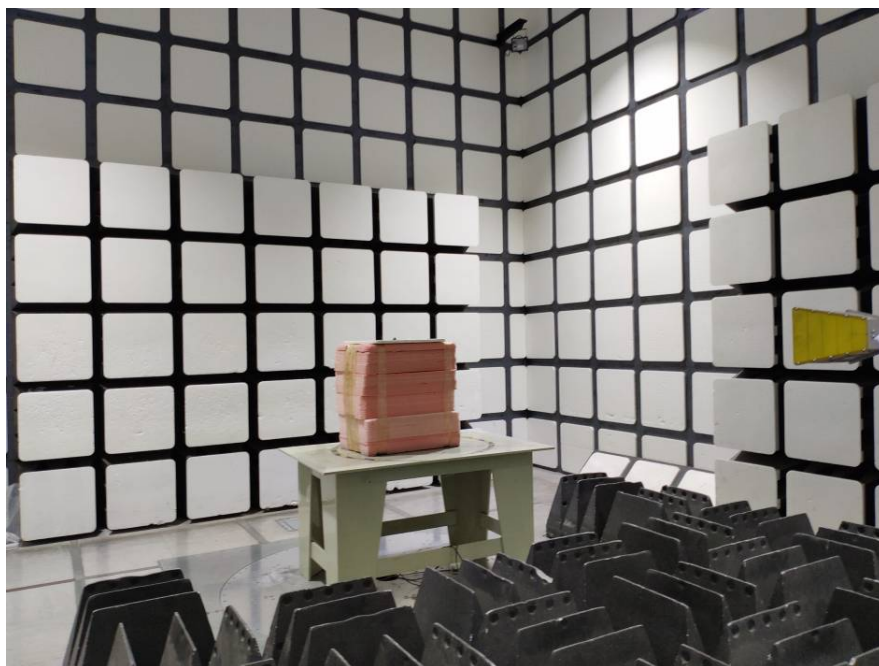
Radiated Emissions View (Above 1 GHz)
