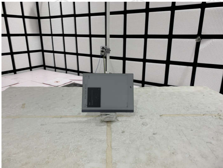
Radiated spurious emission Test Setup-3(Above 1GHz)
