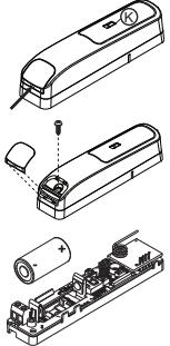
**Note:** When manually programming wireless devices, if a device has been powered up for more than 48 hours it cannot be enrolled into the system until the device has been tampered and restored. When programming the panel using the Quick Enroll procedure follow the steps detailed in Enroll the Device into the System.
