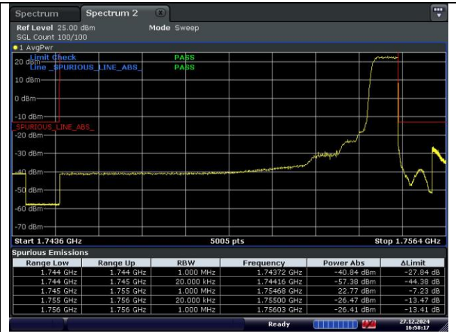
QPSK High Channel - 1 RB - Right
