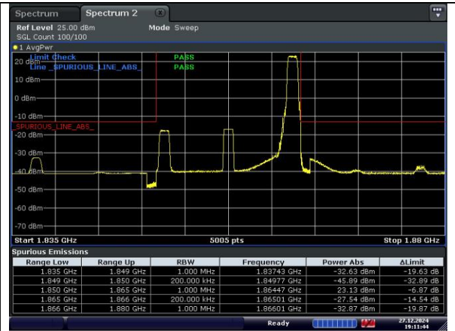
QPSK Low Channel - 1 RB - Right
