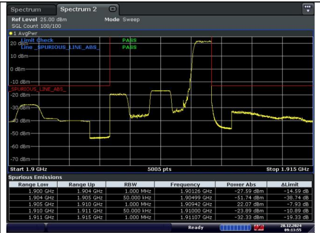
16QAM High Channel - 1 RB - Right
