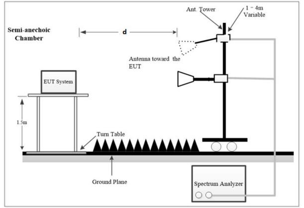
The radiated emission tests using the setup accordance with the ANSI C63.10-2013. The specification used was the FCC 15.209, and FCC 15.247 limits.
