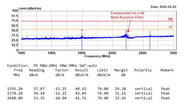
Project No.: 2407A60454E-RF Test Mode: BLE 1M 2440MHz EUT Model: UV-32 Test distance: 3m Temp/Humi/ATM: 21.3°C/49%/100.1kPa Tested by: Wlif Wu Power Source: AC 120V/60Hz
