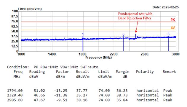
Project No.: 2407A60454E-RF Test Mode: BLE 1M 2480MHz EUT Model: UV-32 Test distance: 3m Temp/Humi/ATM: 21.3°C/49%/100.1kPa Tested by: Wlif Wu Power Source: AC 120V/60Hz
