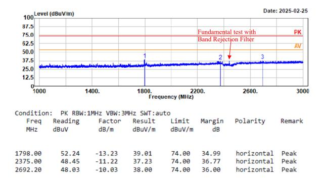
Project No.: 2407A60454E-RF Test Mode: BLE 1M 2440MHz EUT Model: UV-32 Test distance: 3m
