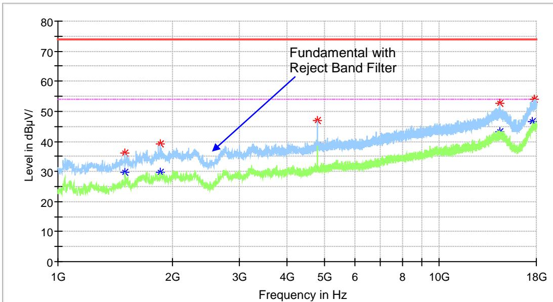
**BDR Mode (GFSK): High Channel \_Vertical\_1GHz-18GHz**
