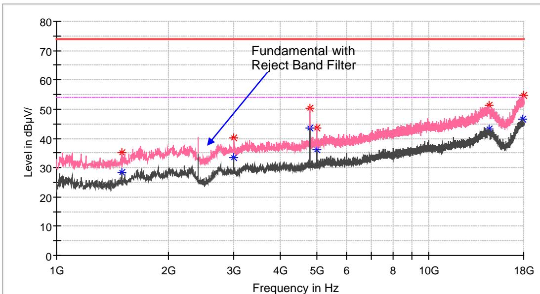
**BDR Mode (GFSK): High Channel \_Horizontal\_18GHz-25GHz**
