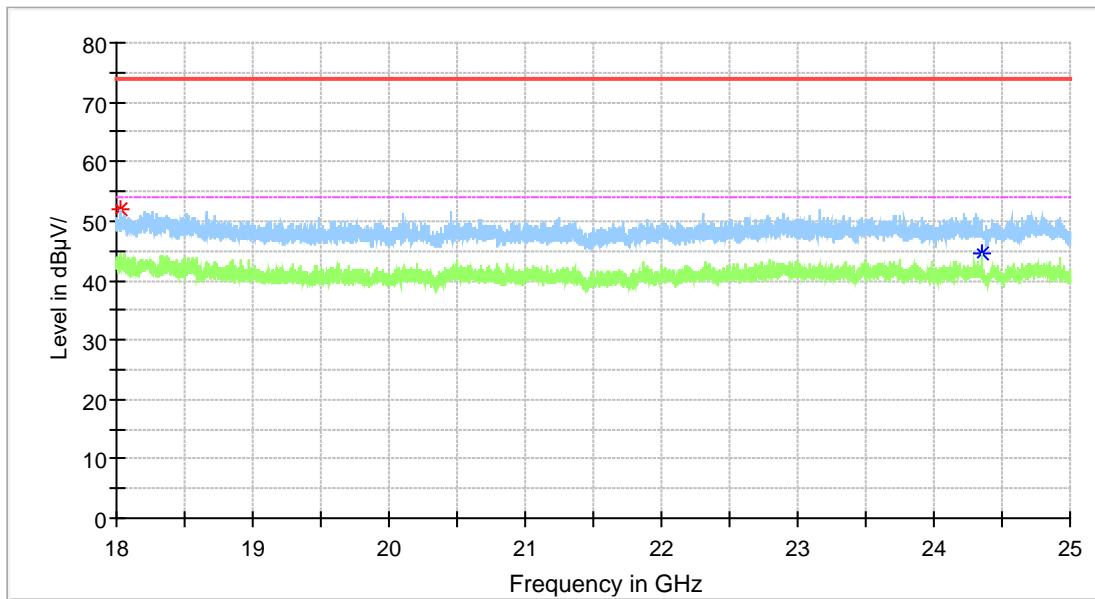
**BDR Mode (GFSK): High Channel \_Vertical\_18GHz-25GHz**
