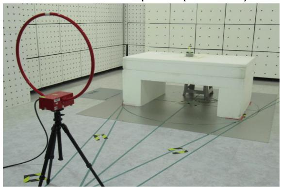
Radiated Emission Set up Photos (Below 1GHz)
