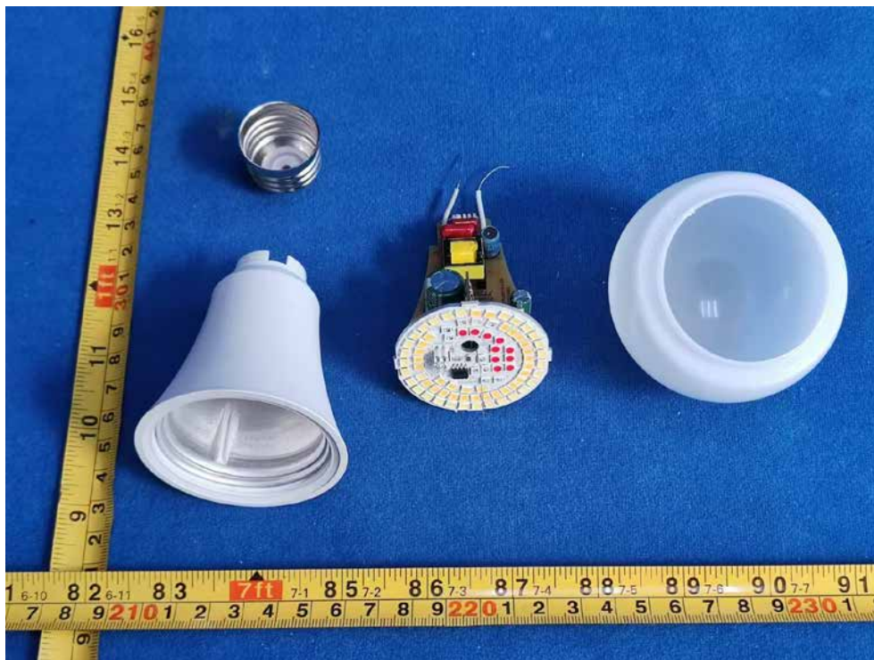
FIGURE 8 DIRECT CONNECT FULL COLOR A21 (M/N: CLEDA2116CDMS) MAINBOARD FRONT
