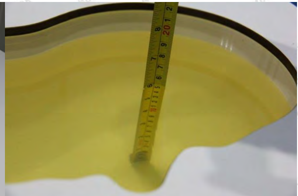
Liquid depth in the Head Phantom (1900MHz)
