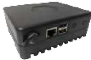
As Trek tabs pass within range, the Gateway will automatically transfer Trek Tab data to your account. The Gateway will continue monitoring the Treks consistently, as long as they are within range, whether they are packed in a shipment or not.
