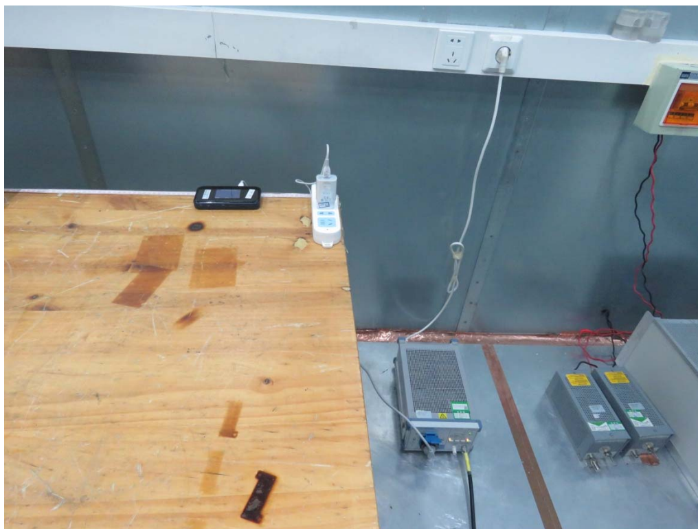
Picture 1: Conducted Emissions Test Setup
