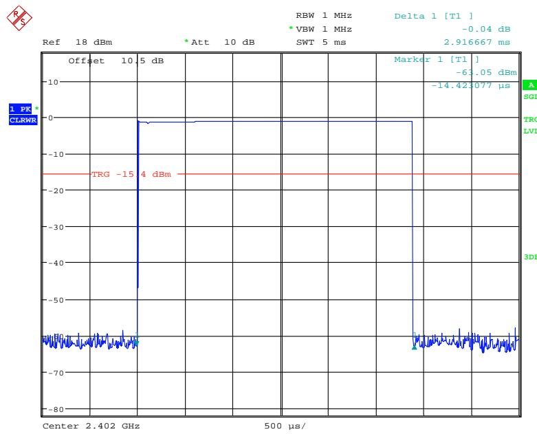
**EDR ( $\pi/4$ -DQPSK):****Pulse time, 2DH1**
