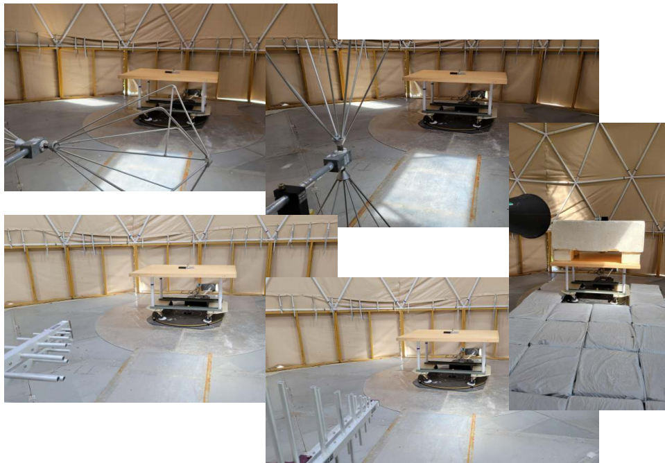
Figure 4.1.1 (v) Radiated Emissions Test Setup Photograph(s).
