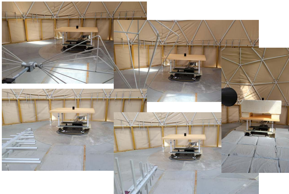
Figure 4.1.1 (ii) Radiated Emissions Test Setup Photograph(s).
