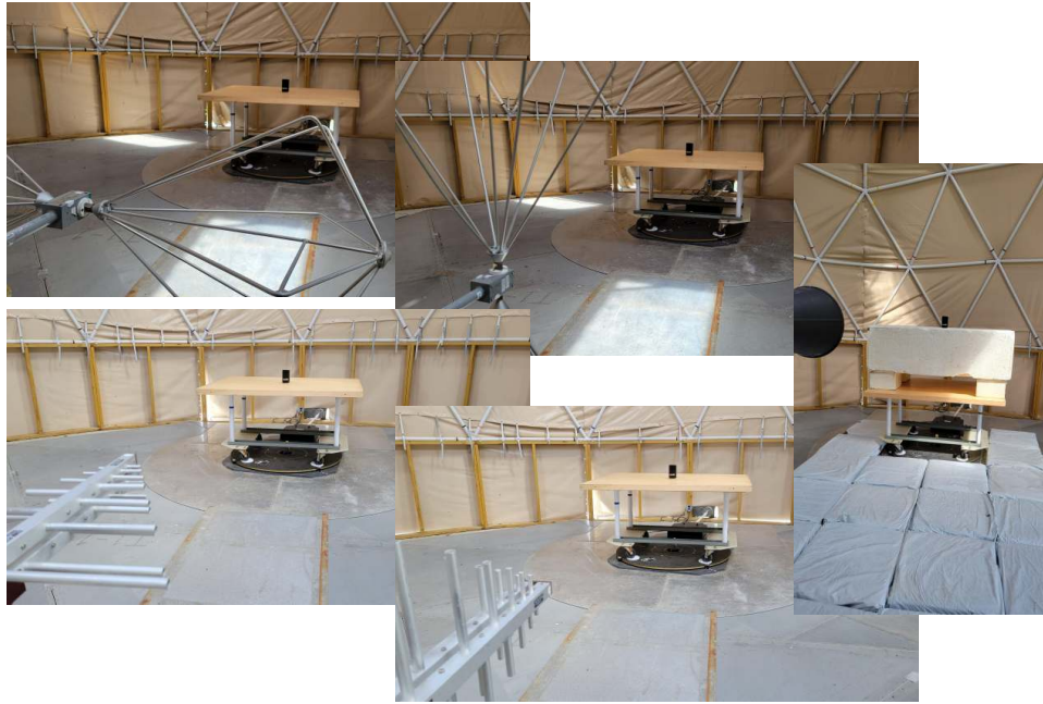
Figure 4.1.1 (i) Radiated Emissions Test Setup Photograph(s).
