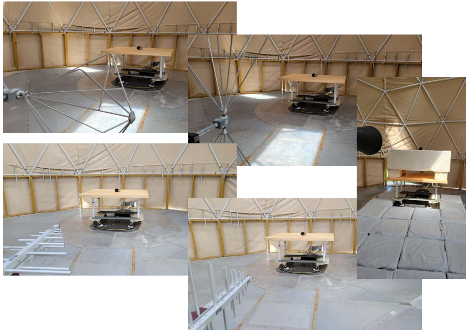
Figure 4.1.1 (iii) Radiated Emissions Test Setup Photograph(s).
