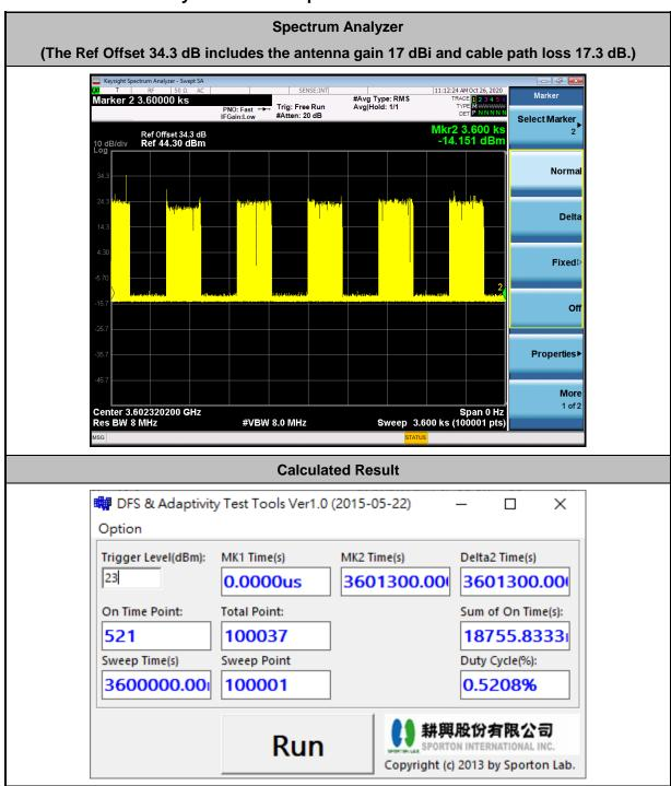
The sum of On Time (aggregated time from marker 1 to 2): 18.75s < 20s, Pass.
