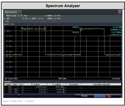
Note: The duty cycle value is 40%, add 10log(1/duty cycle) to the measured power level to compute the average power during continuous transmission.
