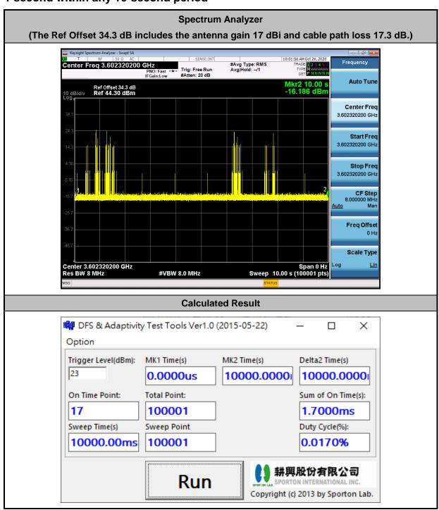
The sum of On Time (aggregated time from marker 1 to 2): 1.7ms < 1s, Pass.
