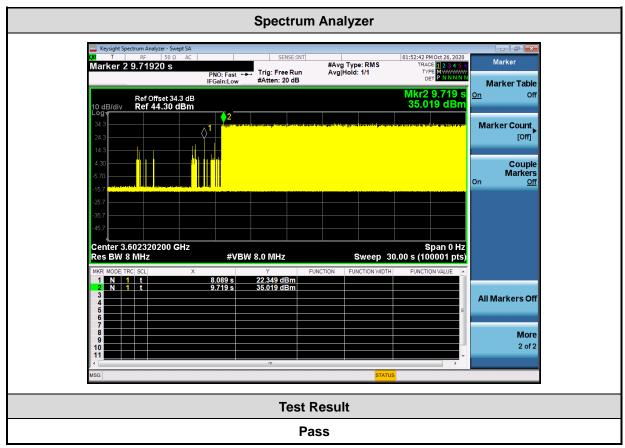
Note: The Ref Offset 34.3 dB includes the antenna gain 17 dBi and cable path loss 17.3 dB.
