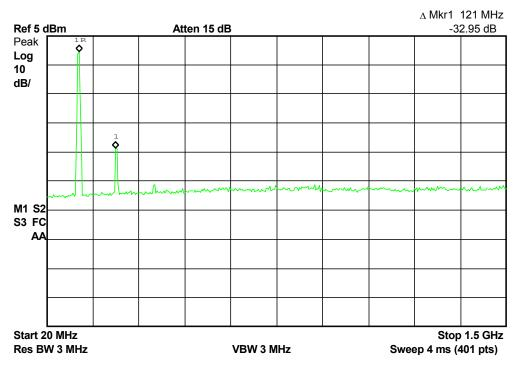
The figure above shows the 121MHz transmitter spectrum. The largest harmonic present is the 2nd harmonic at –32.95dBc.
