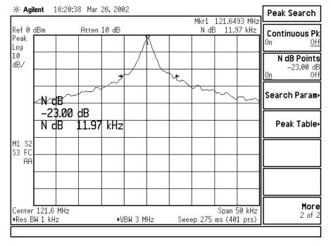
The screen shot above shows that the occupied bandwidth for the 121MHz transmitter, (with A3X modulation), is 11.97kHz.
