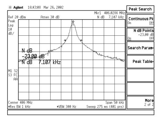
The screen shot above shows that the occupied bandwidth for the 406MHz transmitter is 7.107kHz.
