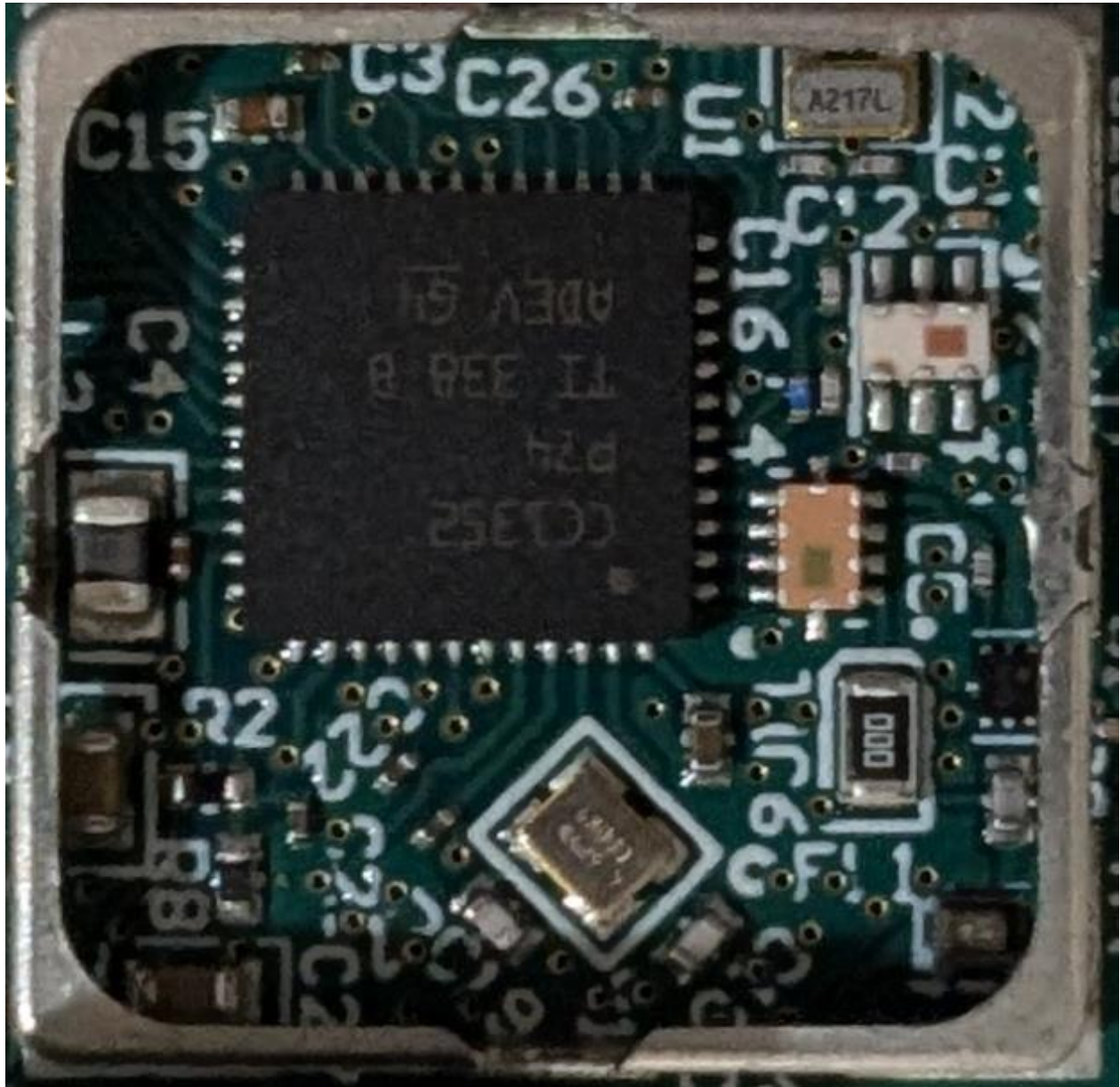
Photograph 1 – Closeup of RF Circuitry Under the Shield
