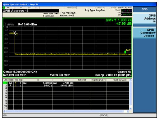
**Verdict:** To verify whether channel is unavailable to be operated in 30 minutes. 1.8ks = 1800s = 1800 s/min /60 = 30minute
