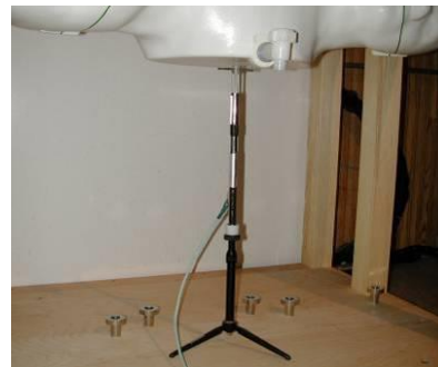
Figure 8-2 System Verification Setup Photo
