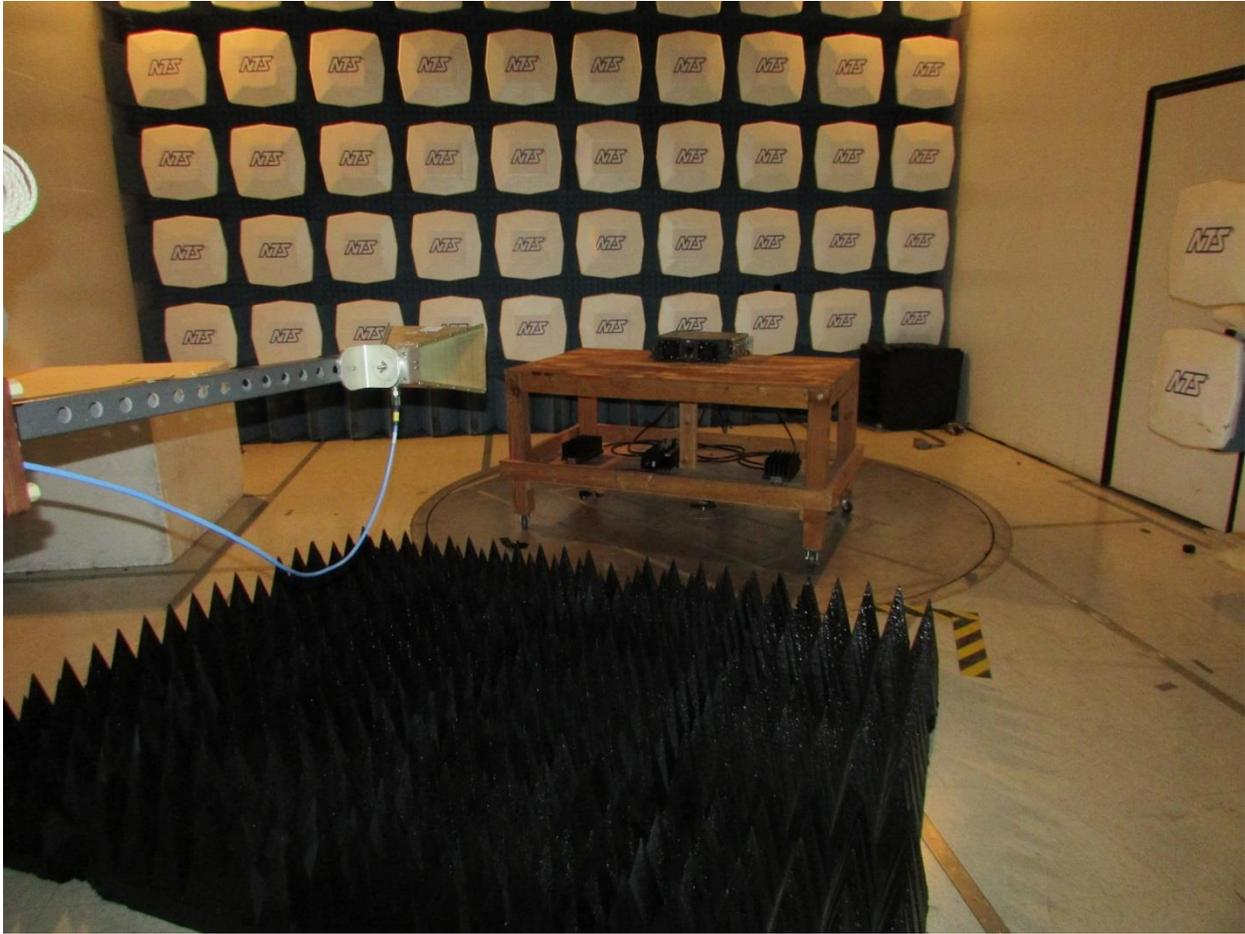
1-18GHz Radiated Measurements
