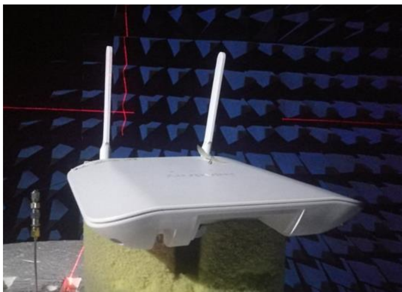
Figure 6 Antenna Device in chamber
