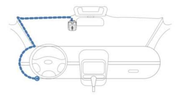
Through the safe box can facilitate the driving recorder to take power, can make it work safely, but also make the recorder line more hidden, the car cloth safe box location: most models of the safe box location in the left side of the driving position or near the steering wheel. Refer to the car instructions for details.
