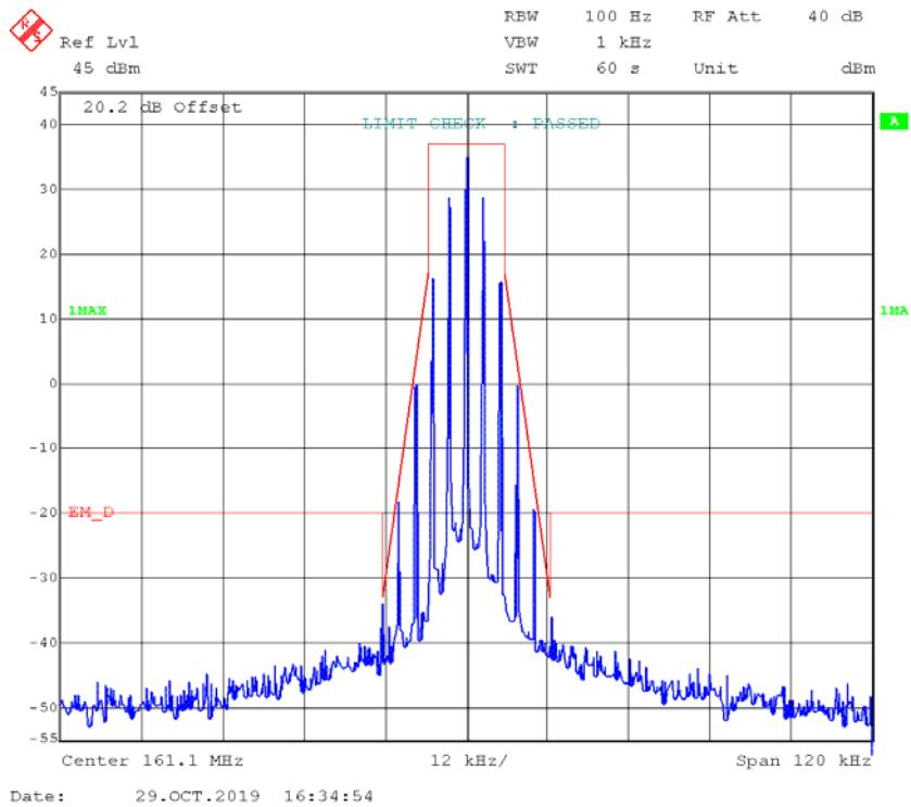
**FM,12.5kHz,Low Power – Frequency 161.1 MHz:****99% Occupied & 26 dB Bandwidth**
