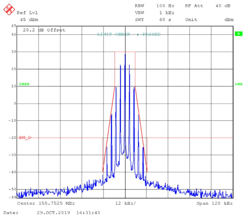
**4FSK,12.5kHz,High Power - Frequency 155.7525 MHz:****99% Occupied & 26 dB Bandwidth**
