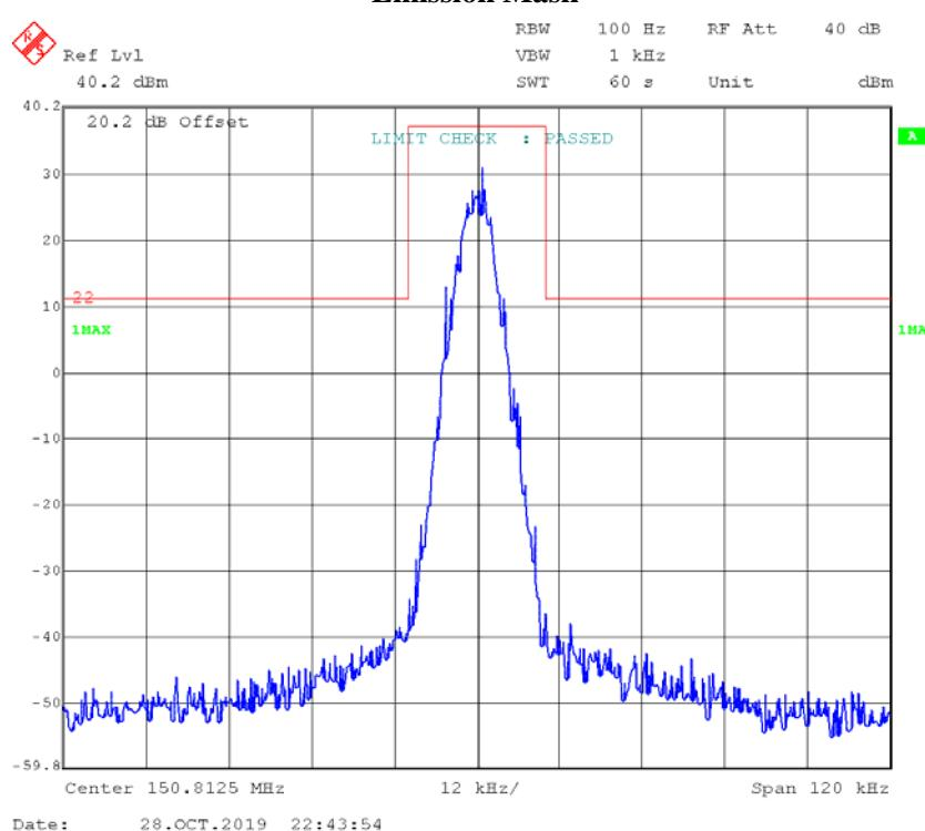
**4FSK,12.5kHz,Low Power - Frequency 150.8125 MHz:****99% Occupied & 26 dB Bandwidth**
