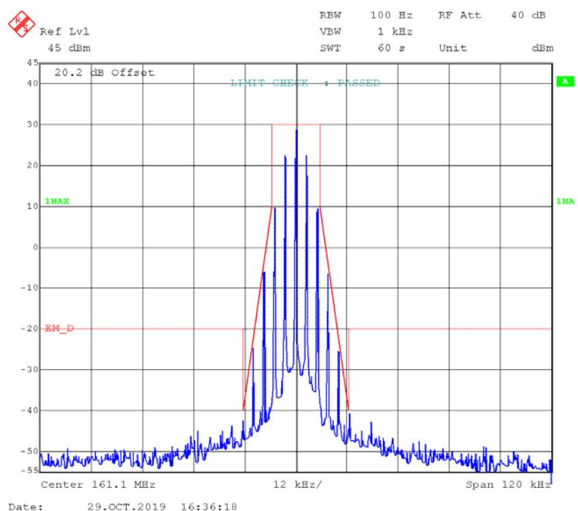
**FM,25kHz,High Power - Frequency 161.1 MHz****: 99% Occupied & 26 dB Bandwidth**
