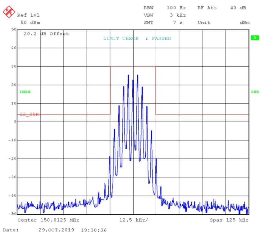
**4FSK,12.5kHz,High Power - Frequency 150.8125 MHz:****99% Occupied & 26 dB Bandwidth**
