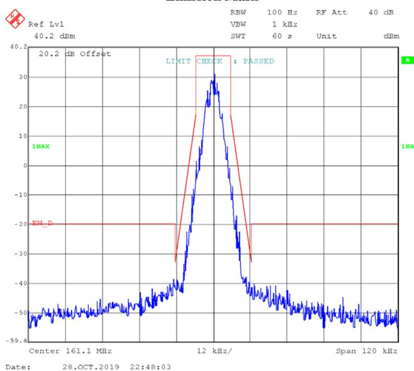
**4FSK ,12.5kHz, Low Power - Frequency161.1 MHz:****99% Occupied & 26 dB Bandwidth**
