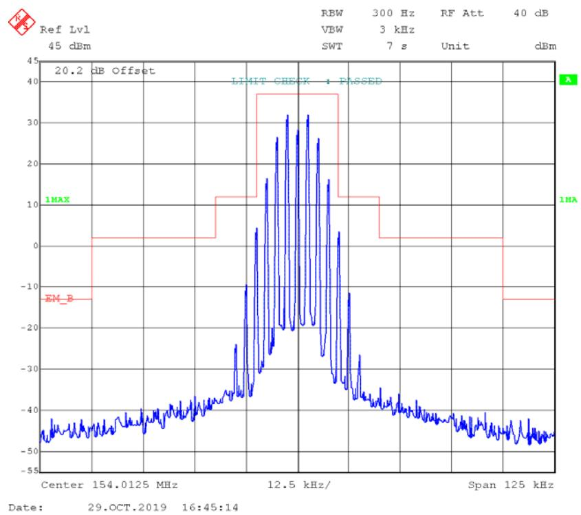
**FM,25kHz,Low Power - Frequency 154.0125 MHz:****99% Occupied & 26 dB Bandwidth**
