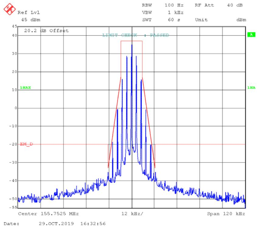
**FM,12.5kHz,Low Power - Frequency 155.7525 MHz:****99% Occupied & 26 dB Bandwidth**
