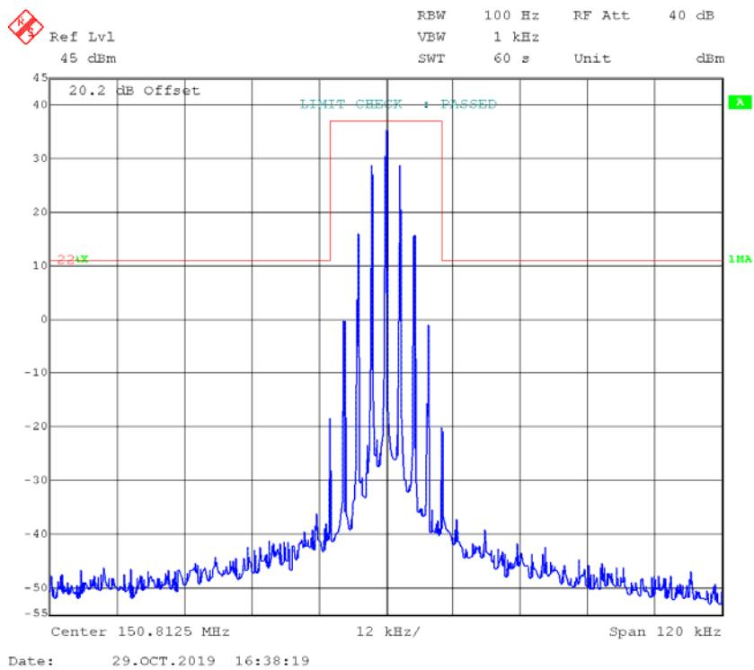
**FM,12.5kHz,Low Power - Frequency 150.8125 MHz:****99% Occupied & 26 dB Bandwidth**
