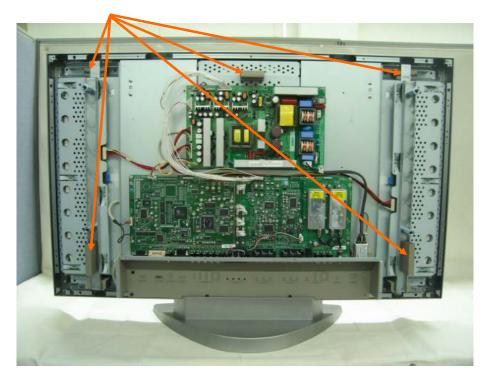
2. Apply a ferrite Core to the Speaker Cable and LVDS Cable
