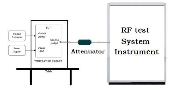
5.1.2 Slave and Client device(EUT) block diagram of Test setup
