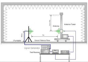
Test Setup for Above 1 GHz
