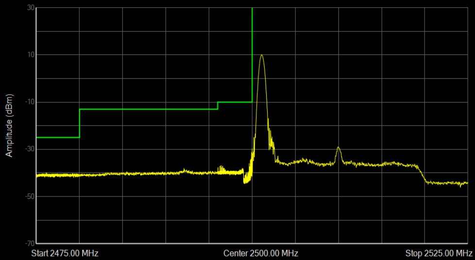
Band7 16QAM BW=20MHz Channel=20850 RB Size=1 Position=#0
