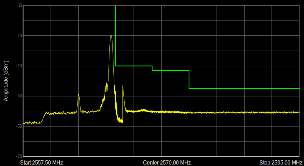
Band7 QPSK BW=10MHz Channel=21400 RB Size=1 Position=#Max
