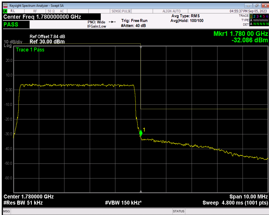
Band66 QPSK BW=10MHz Channel=132022 RB Size=1 Position=#0
