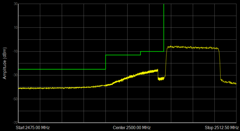
Band7 16QAM BW=10MHz Channel=20800 RB Size=50 Position=#0
