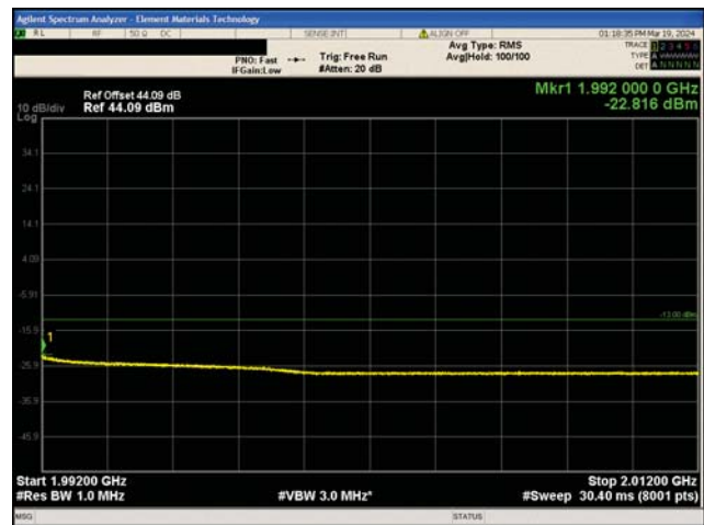
2G GSM/EDGE Band 2 Test Case 3 8PSK Modulation Upper Band Edge
