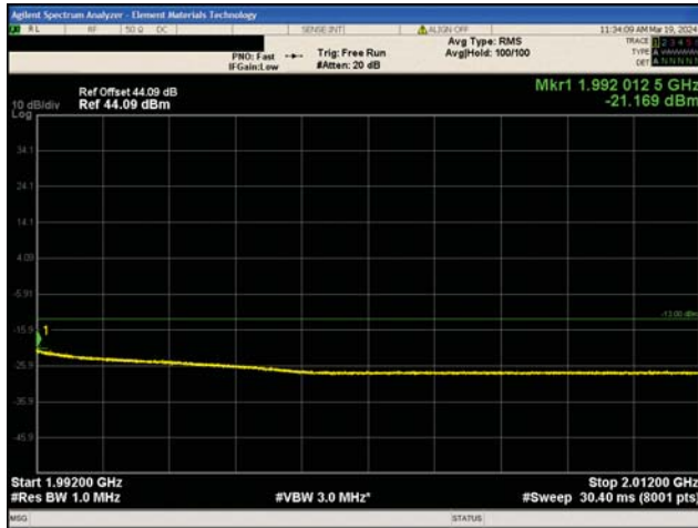
2G GSM/EDGE Band 2 Test Case 2 GMSK Modulation Upper Band Edge
