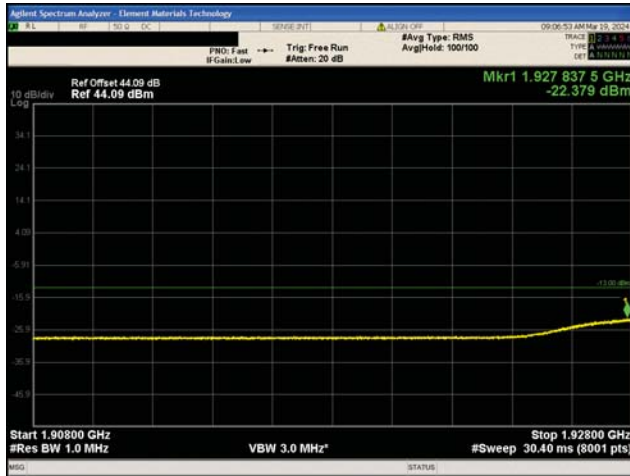
2G GSM/EDGE Band 2 8PSK Modulation One Channel Inside Low Channel, 1930.4 MHz
