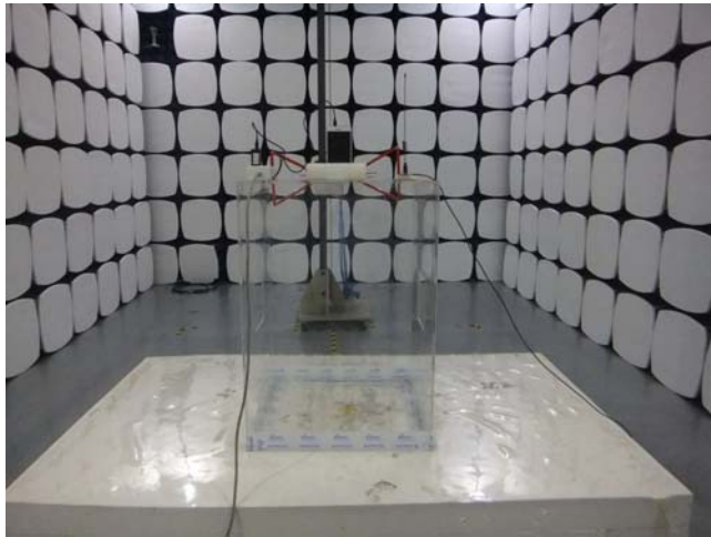
Radiated Spurious Emissions Test Setup Below 1GHz
