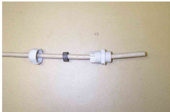
Step 1: Assemble gland on cable as shown
