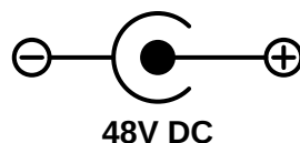
Figure 30 DC Connection Diagram
