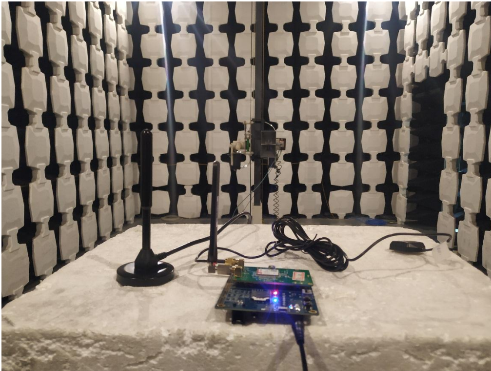
Radiated Spurious Emission Test Setup photo (the frequency above 3000MHz)
