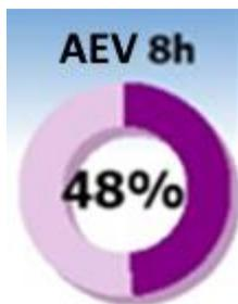
The AEV donut displays 48%, which corresponds to the ratio of the average of samples taken over the last 8 hours to the value configured in the "TWA Customization" menu.
