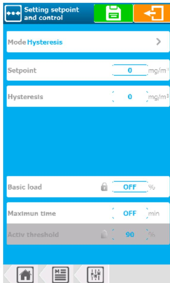
**When the dosing direction of the channel is configured in descending mode**, as soon as the error (measurement – setpoint) is greater than the hysteresis value the need for regulation is 100%.
