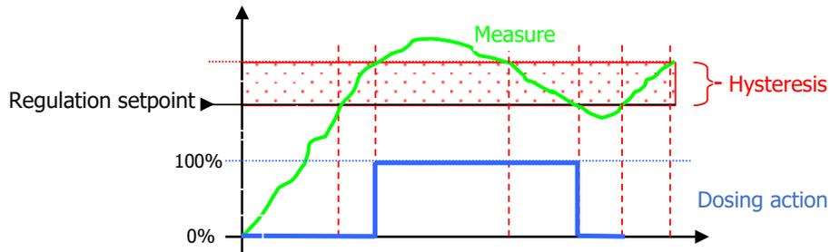
**When the dosing direction of the track is configured in ascending mode**, as soon as the error (setpoint – measurement) is greater than the hysteresis value the need for regulation is 100%.
