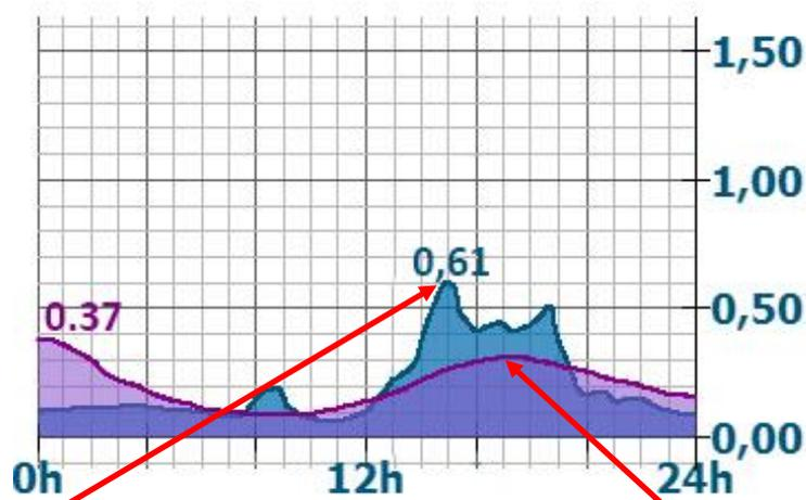
At 3pm, the ELV (i.e. the average of samples taken over the last 15 minutes) is 0.61mg/m<sup>3</sup>
