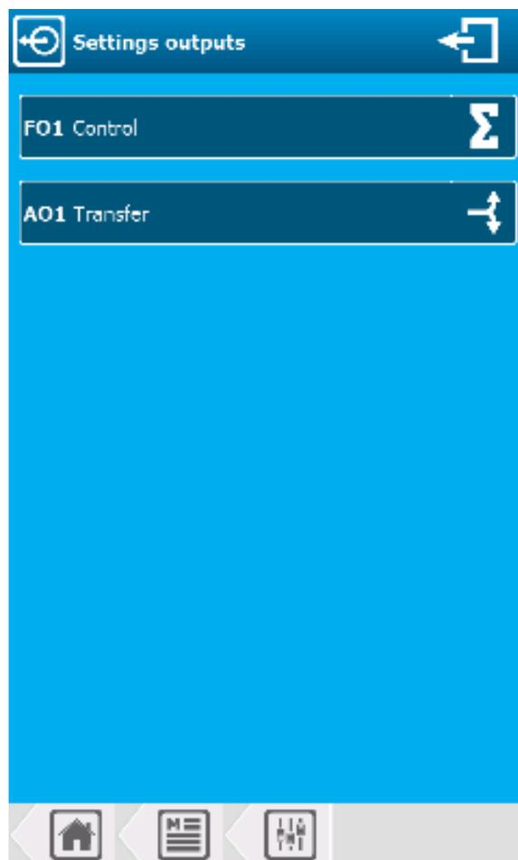
The screen shows which outputs are already configured and which are not in use. Pressing an output that is already set, you can modify its configuration, or pressing an unused output, you can configure its installation.
