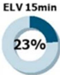
The ELV donut displays 23%, which corresponds to the ratio between the average of samples taken over the last 15 minutes and the value configured in the "Customize ELV" menu.
