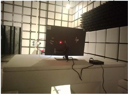
Radiated Emission Set up Photos (30MHz~1GHz)
