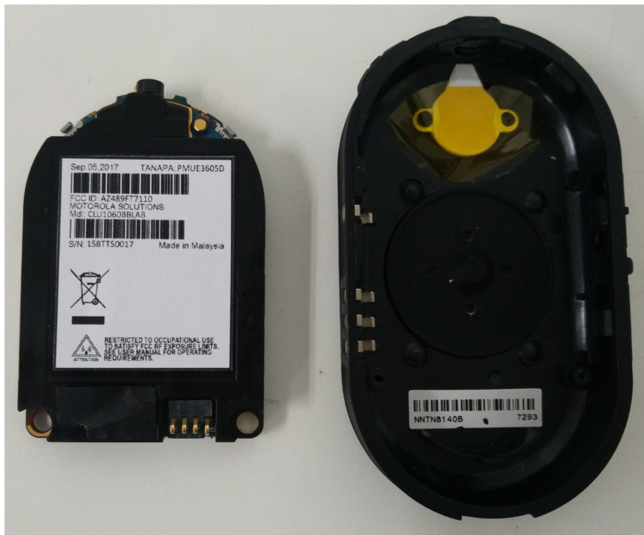
Chassis and Housing (Back side) (CLP1060, CLP1063)
