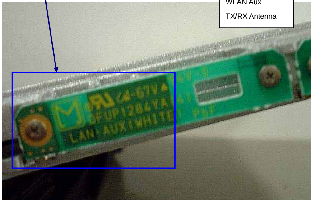
WLAN Aux TX/RX Antenna
