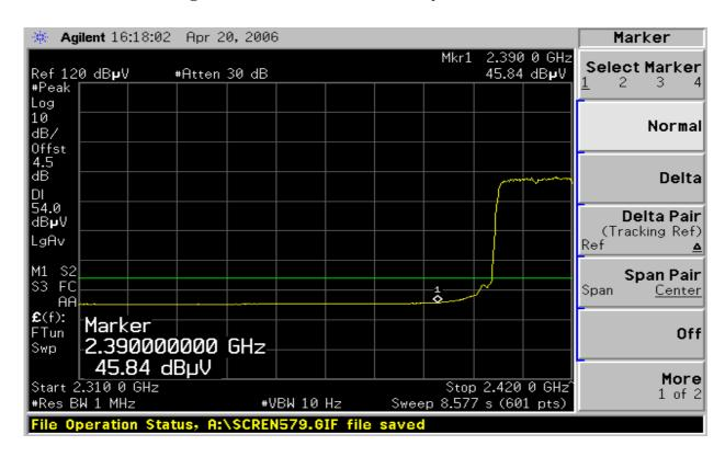
Detector mode: Peak Polarity: Horizontal
