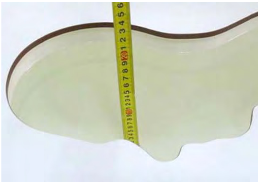
Picture 9: Liquid depth in the head Phantom (2600 MHz, 15.4cm depth)
