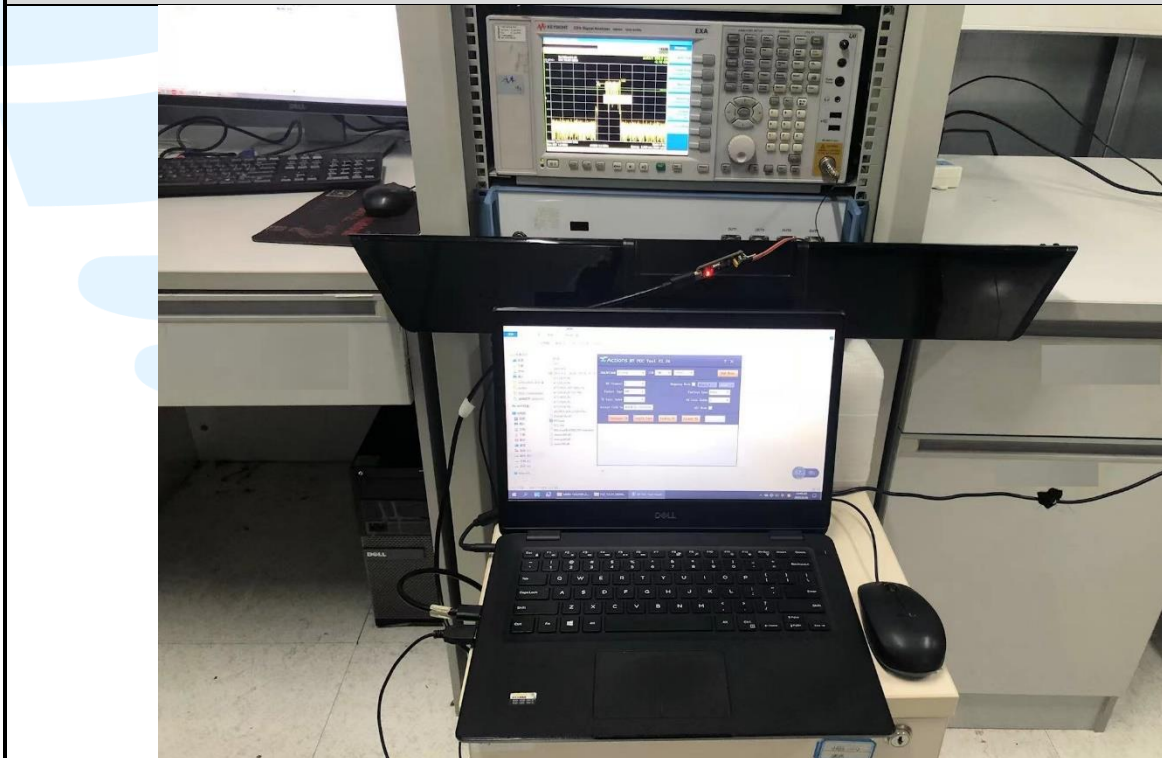
RF Conducted Test Setup
