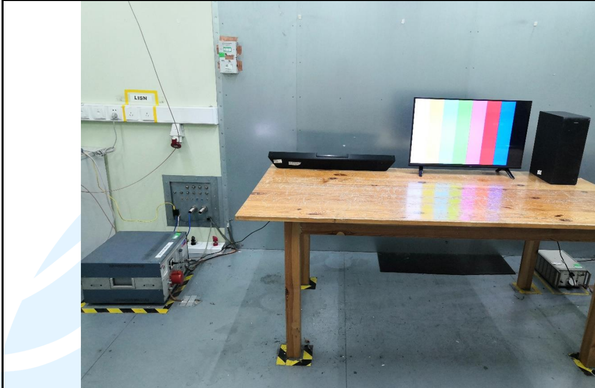
AC Power Line Conducted Emission Test Setup
