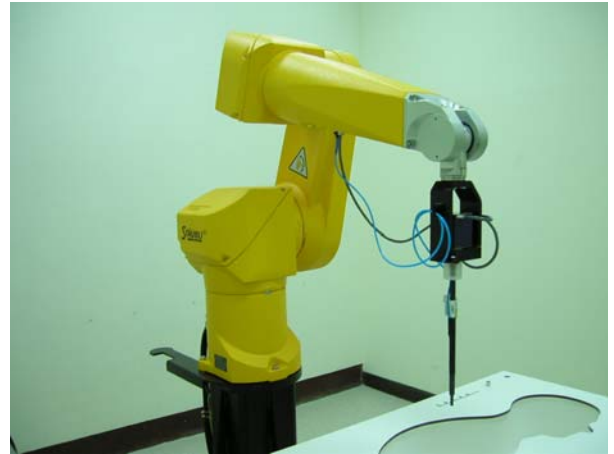
Fig. 5.2 Probe setup on robot
