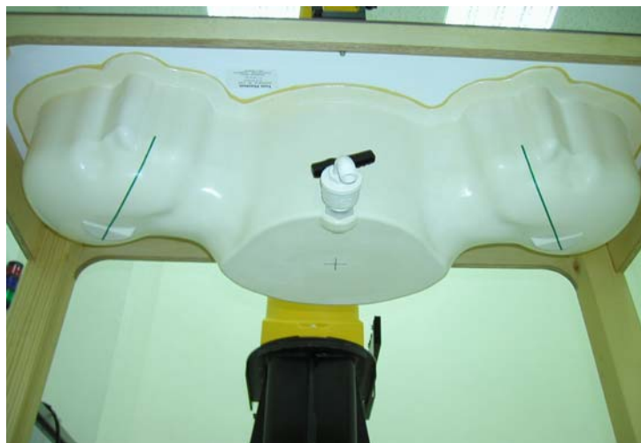
Fig. 5.4 Bottom view of twin phantom
