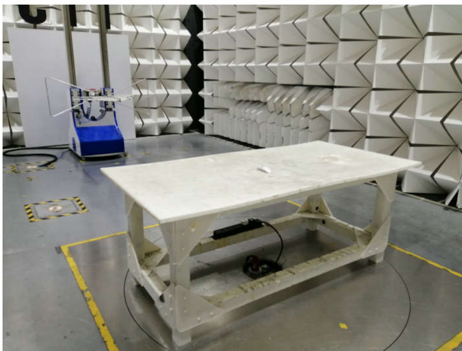
Radiated spurious emission Test Setup-2(30MHz-1GHz)
