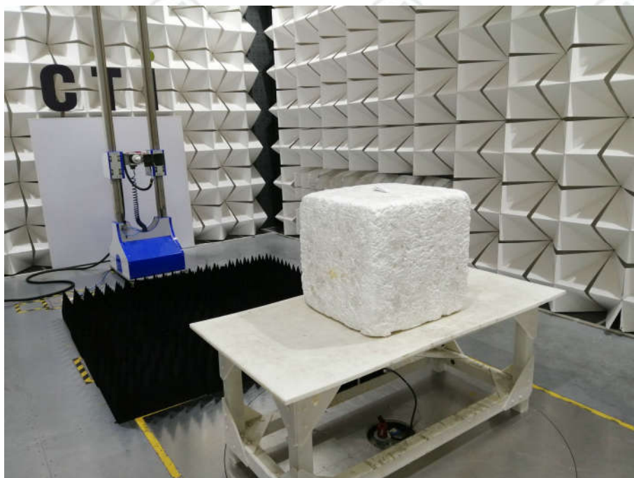
Radiated spurious emission Test Setup-3(Above 1GHz)
