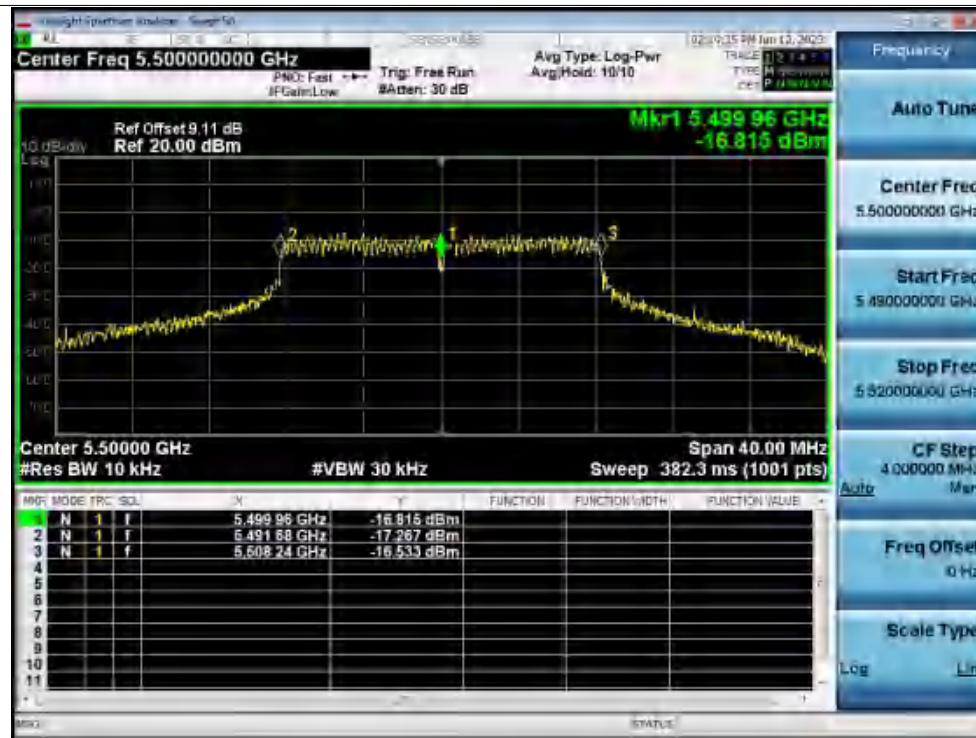
Freq. Stability 50C 120V a 5500MHz Ant1 0 Minutes
