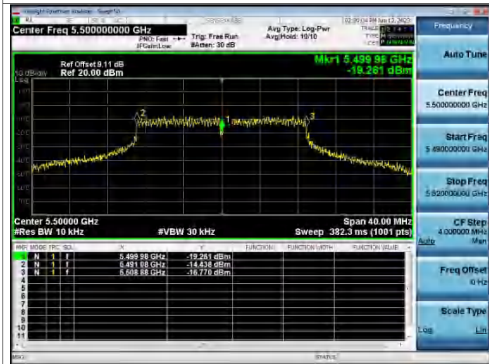
Freq. Stability -20C 120V ac20 5500MHz Ant1 0 Minutes
