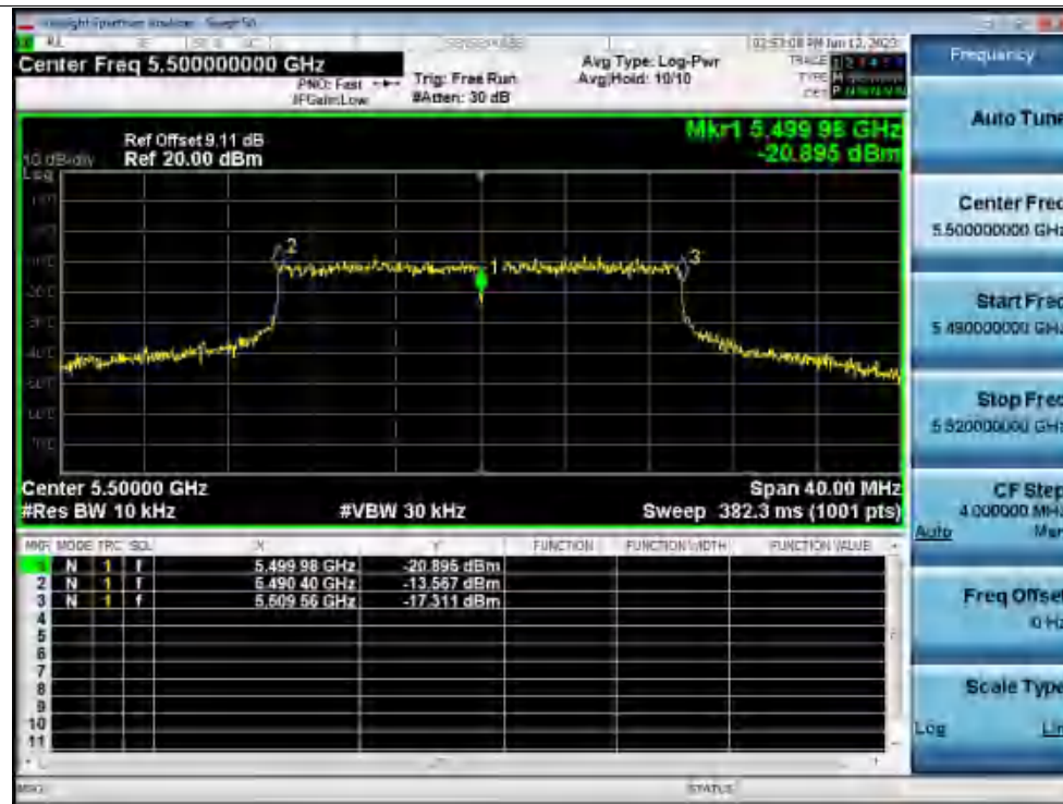
Freq. Stability 0C 120V ax20 5500MHz Ant1 0 Minutes
