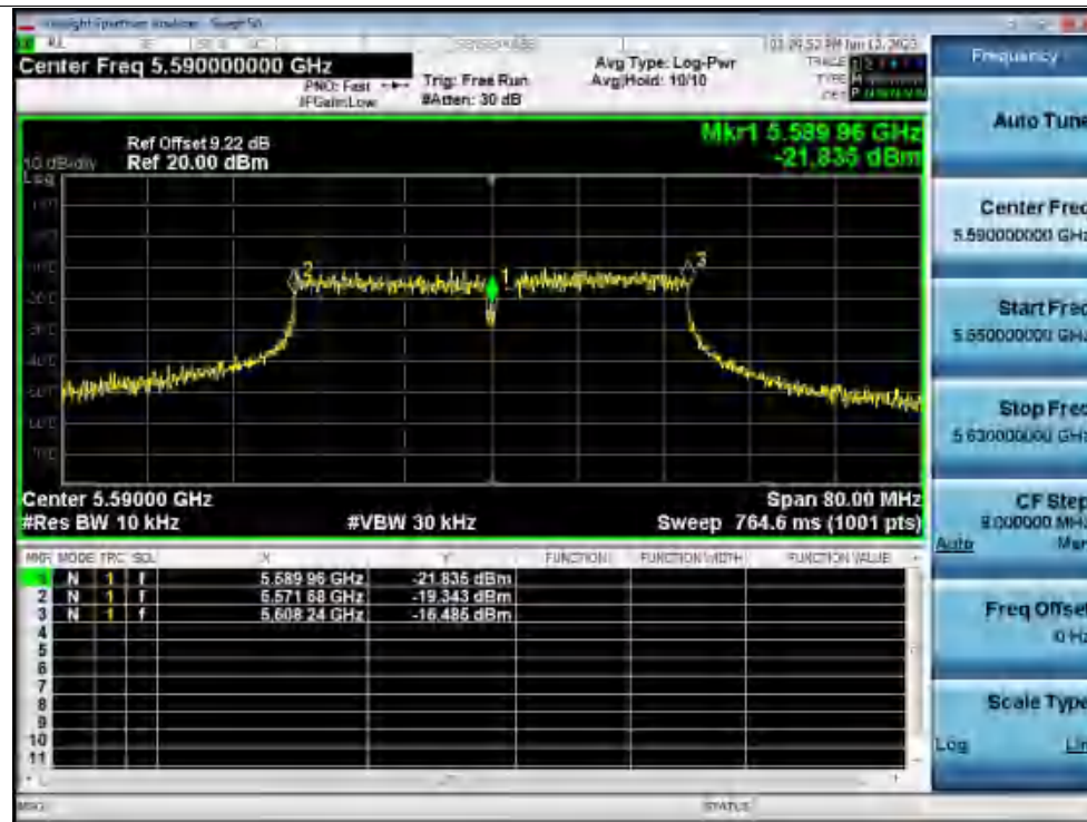
Freq. Stability 30C 120V ac40 5590MHz Ant1 0 Minutes
