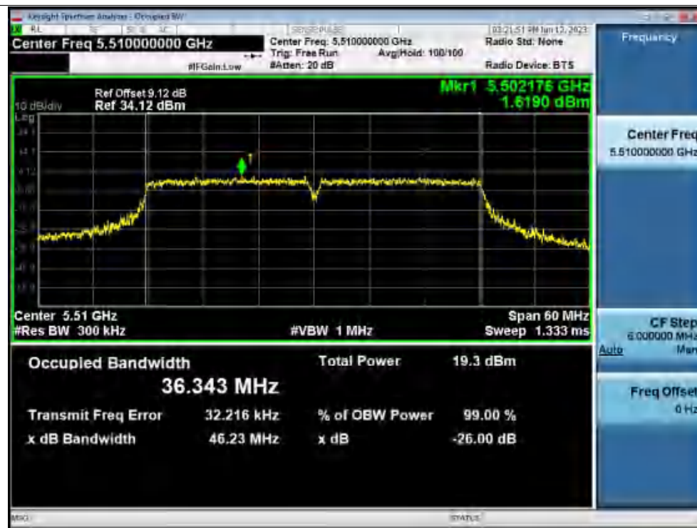
-26dB Bandwidth NVNT ac40 5510MHz Ant1
