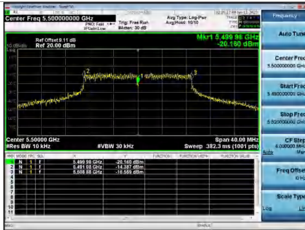
Freq. Stability 30C 120V n20 5500MHz Ant1 0 Minutes
