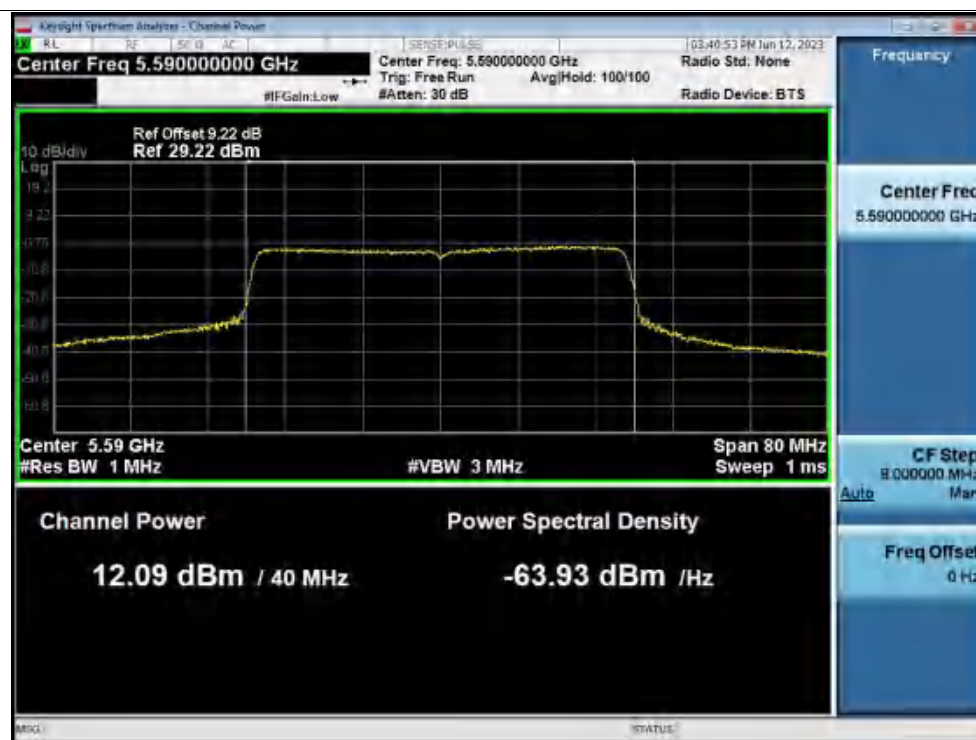
Power NVNT ax40 5590MHz Ant1
