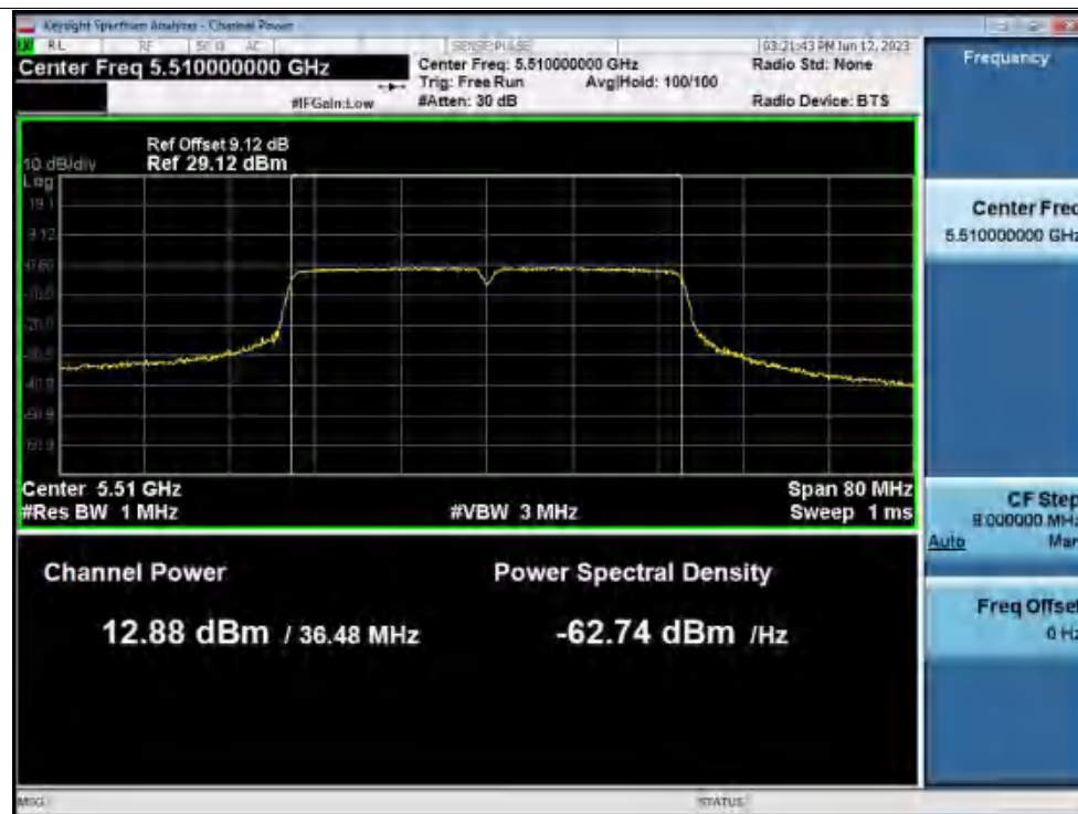
Power NVNT ac40 5510MHz Ant1
