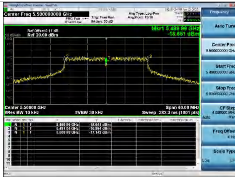
Freq. Stability 20C 120V n20 5500MHz Ant1 0 Minutes
