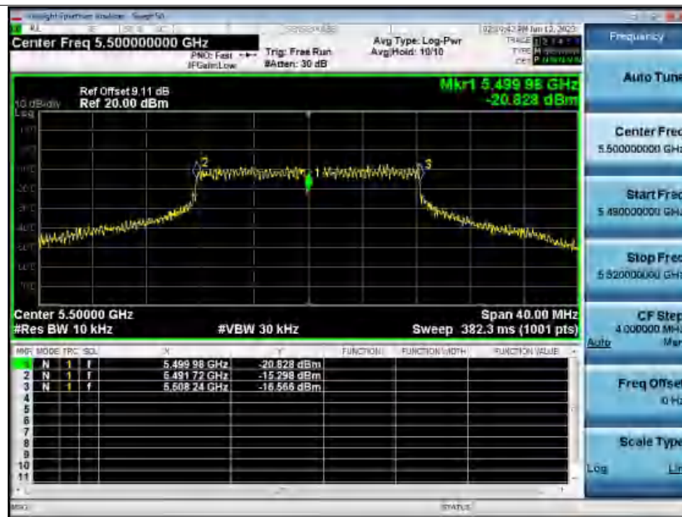
Freq. Stability 50C 120V a 5500MHz Ant1 0 Minutes
