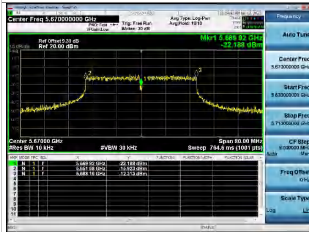
Freq. Stability 50C 120V ac40 5670MHz Ant1 0 Minutes
