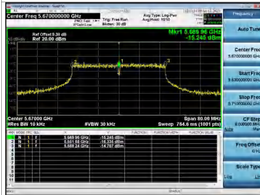
Freq. Stability -20C 120V n40 5670MHz Ant1 0 Minutes
