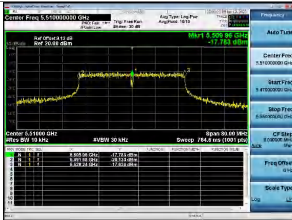
Freq. Stability -20C 120V n40 5510MHz Ant1 0 Minutes
