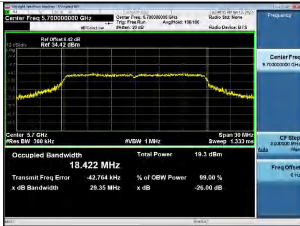
-26dB Bandwidth NVNT ac40 5510MHz Ant1
