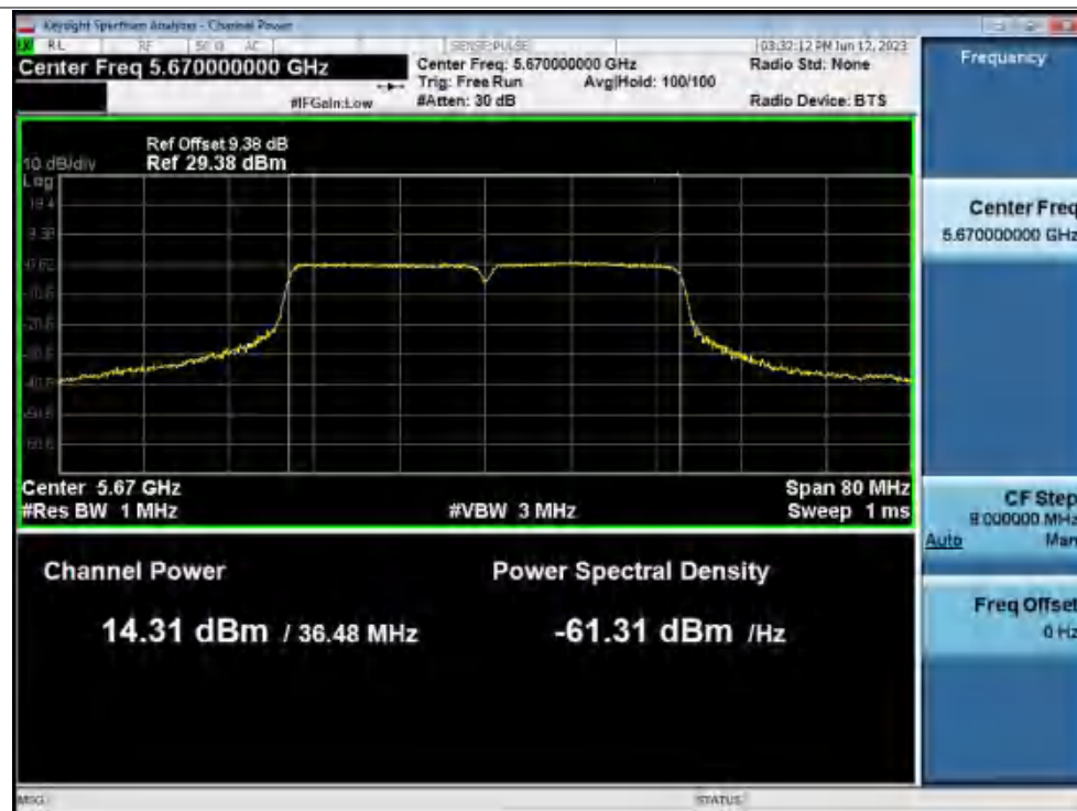
Power NVNT ac40 5670MHz Ant1
