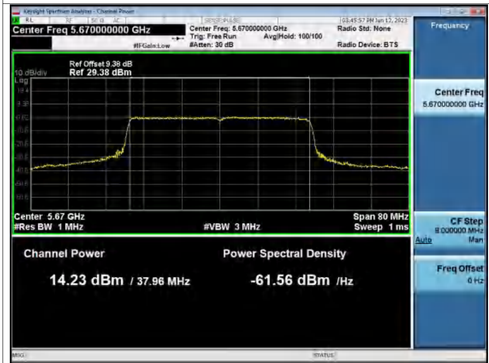
Power NVNT ax40 5670MHz Ant1
