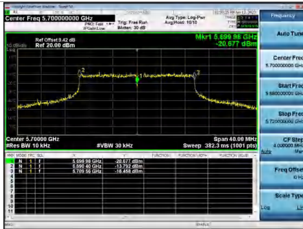
Freq. Stability 0C 120V ax20 5700MHz Ant1 0 Minutes
