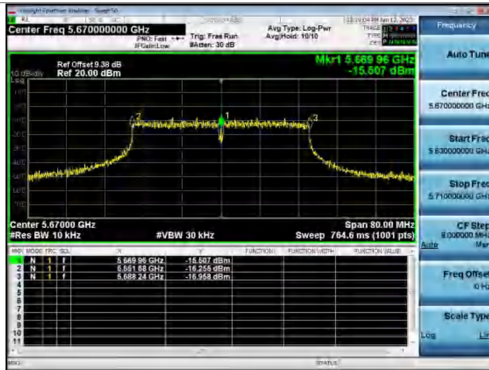
Freq. Stability -20C 120V n40 5670MHz Ant1 0 Minutes
