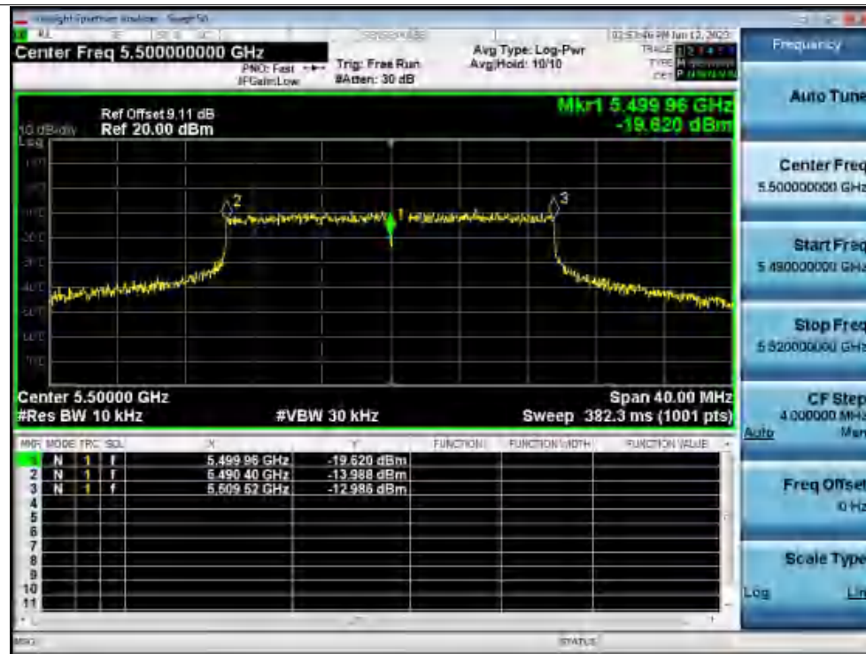
Freq. Stability 50C 120V ax20 5500MHz Ant1 0 Minutes
