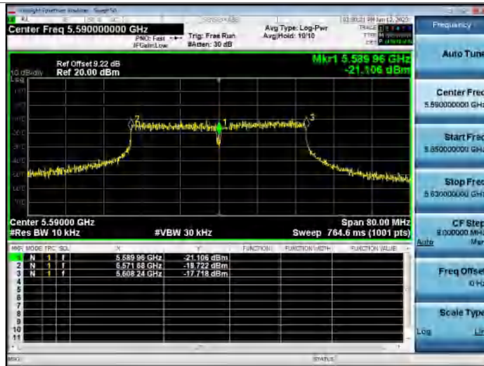
Freq. Stability 50C 120V ac40 5590MHz Ant1 0 Minutes
