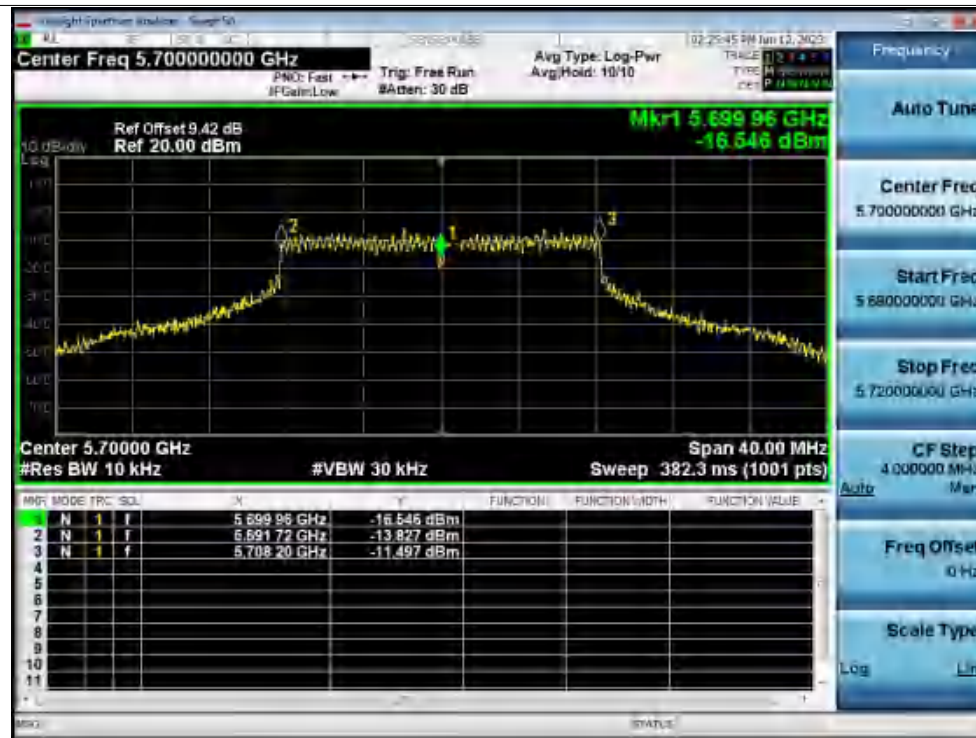
Freq. Stability 0C 120V a 5700MHz Ant1 0 Minutes
