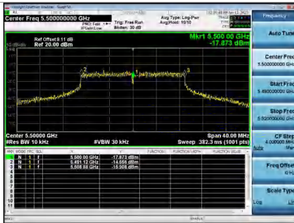
Freq. Stability 50C 120V ac20 5500MHz Ant1 0 Minutes
