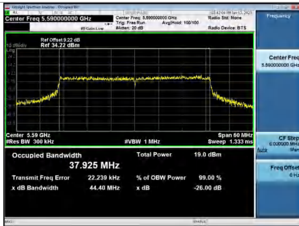
-26dB Bandwidth NVNT ax40 5590MHz Ant1
