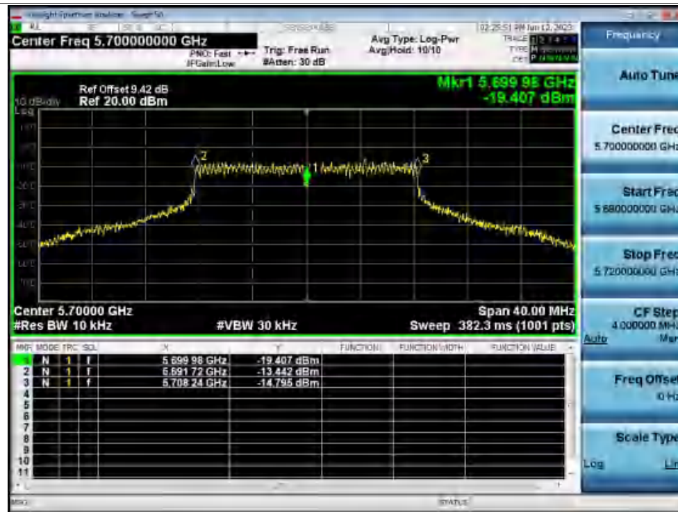
Freq. Stability 0C 120V a 5700MHz Ant1 0 Minutes
