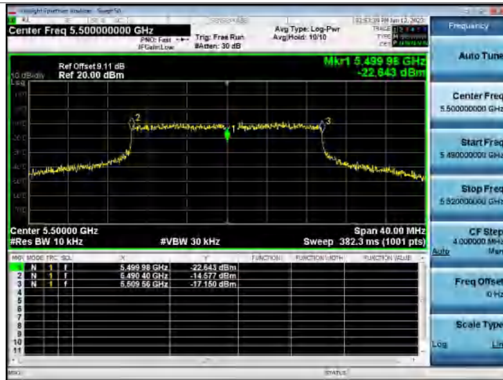
Freq. Stability 50C 120V ax20 5500MHz Ant1 0 Minutes
