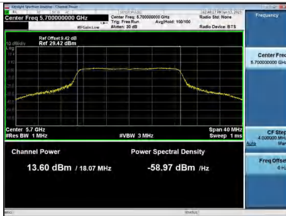
Power NVNT ac40 5510MHz Ant1
