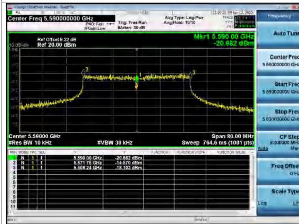
Freq. Stability -20C 120V ac40 5590MHz Ant1 0 Minutes
