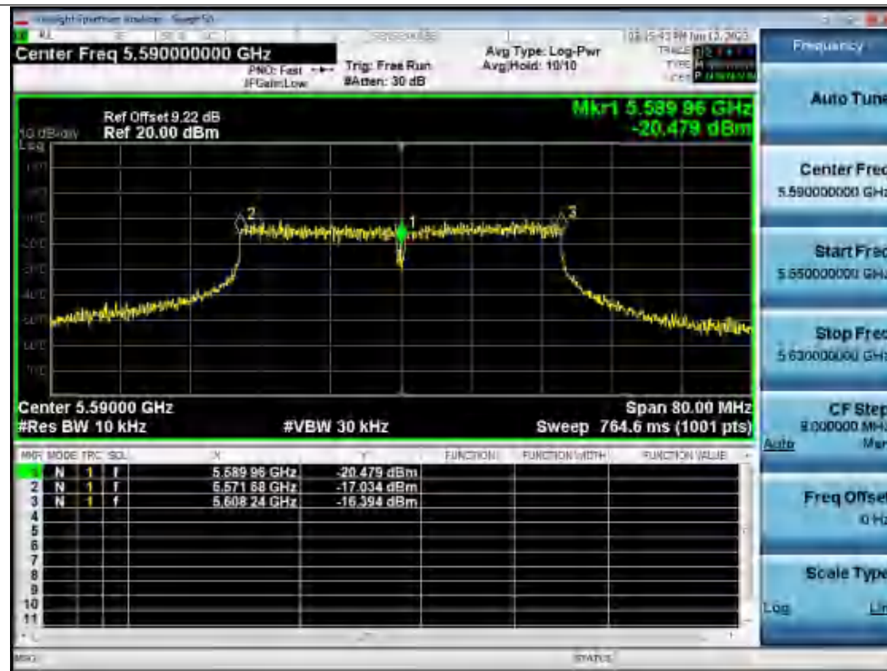
Freq. Stability 30C 120V n40 5590MHz Ant1 0 Minutes
