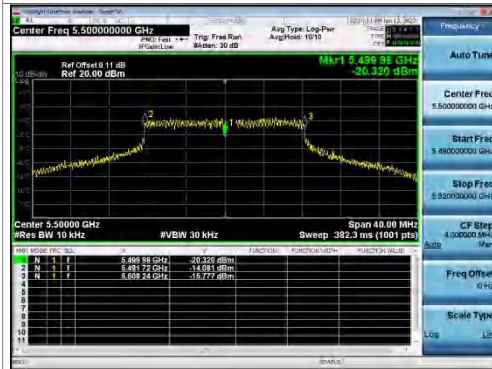
Freq. Stability 0C 120V a 5500MHz Ant1 0 Minutes
