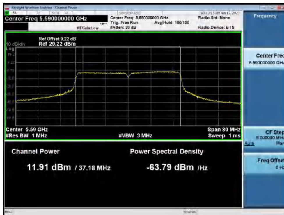
Power NVNT n40 5590MHz Ant1
