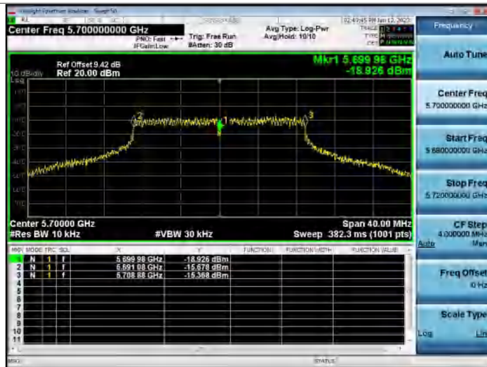
Freq. Stability 20C 102V ac20 5700MHz Ant1 0 Minutes
