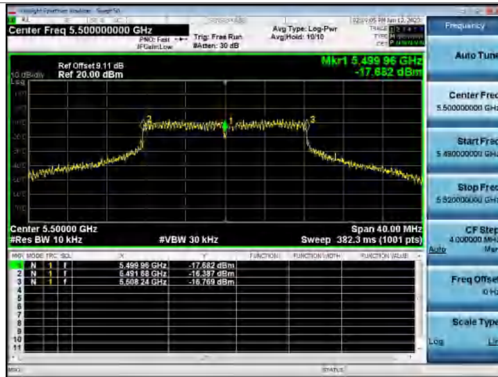
Freq. Stability 0C 120V a 5500MHz Ant1 0 Minutes
