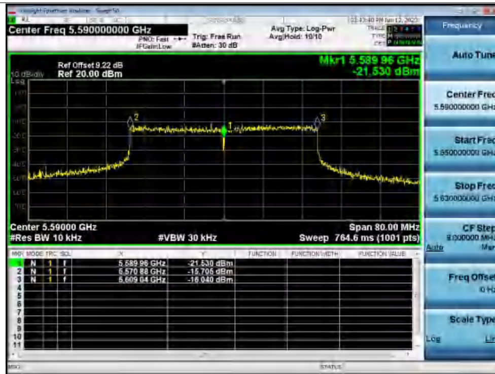
Freq. Stability 30C 120V ax40 5590MHz Ant1 0 Minutes
