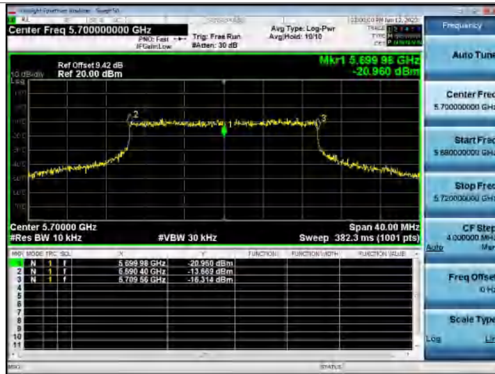
Freq. Stability 30C 120V ax20 5700MHz Ant1 0 Minutes
