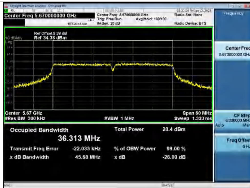
-26dB Bandwidth NVNT ac40 5670MHz Ant1
