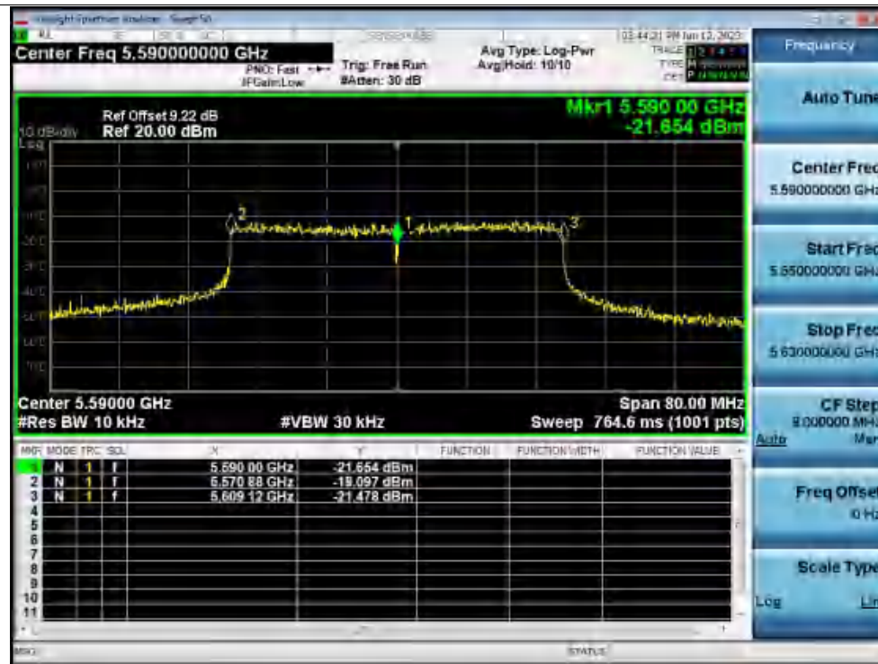
Freq. Stability 50C 120V ax40 5590MHz Ant1 0 Minutes
