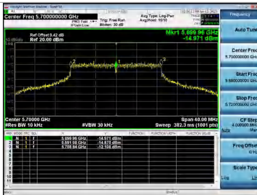
Freq. Stability 20C 120V n20 5700MHz Ant1 0 Minutes
