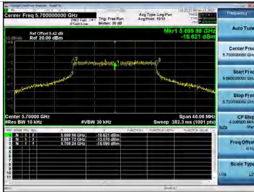
Freq. Stability -20C 120V a 5700MHz Ant1 0 Minutes
