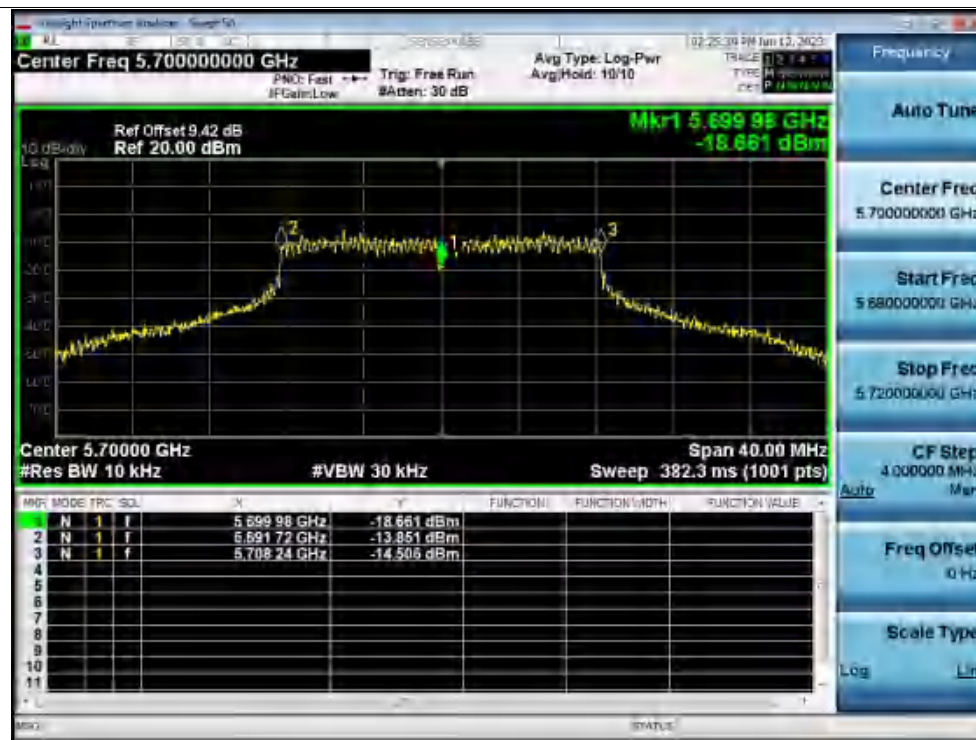
Freq. Stability -20C 120V a 5700MHz Ant1 0 Minutes
