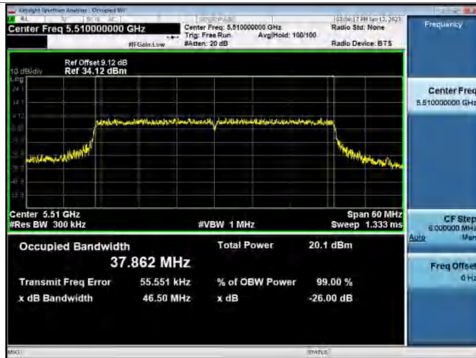
-26dB Bandwidth NVNT ax40 5590MHz Ant1
