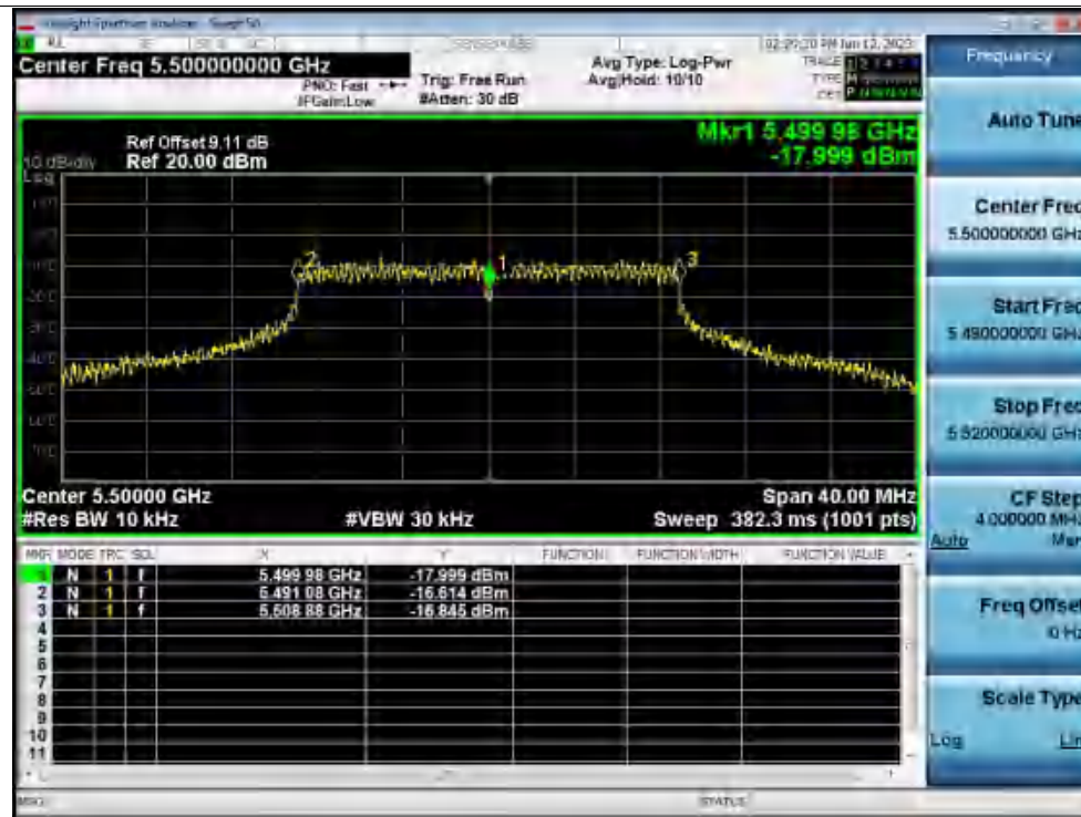
Freq. Stability 30C 120V n20 5500MHz Ant1 0 Minutes
