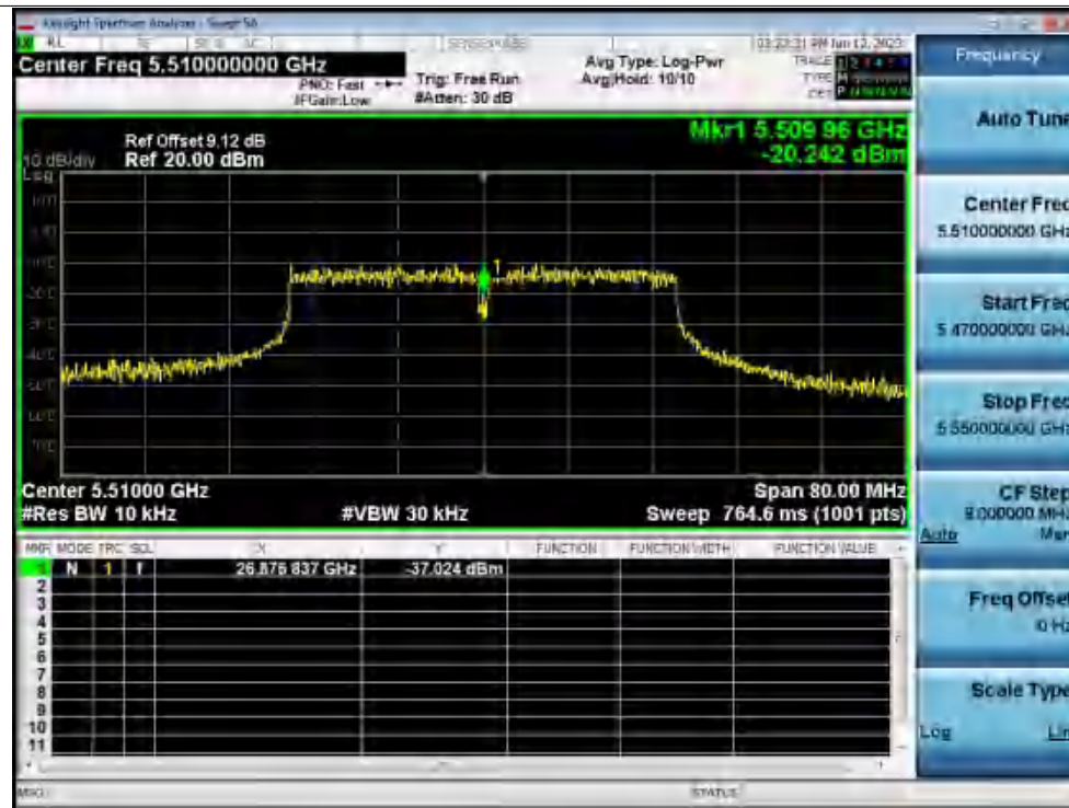
Freq. Stability 20C 120V ac40 5510MHz Ant1 0 Minutes
