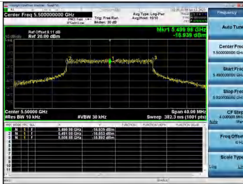
Freq. Stability 0C 120V ac20 5500MHz Ant1 0 Minutes
