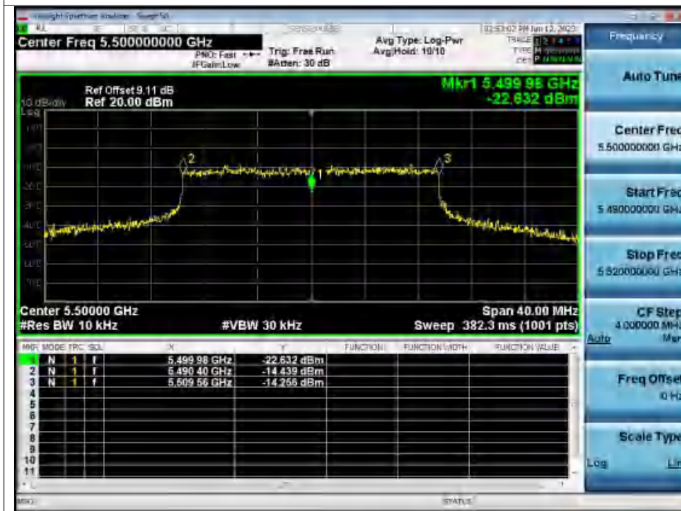
Freq. Stability -20C 120V ax20 5500MHz Ant1 0 Minutes
