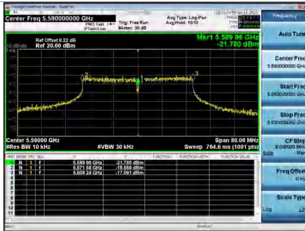
Freq. Stability 30C 120V n40 5590MHz Ant1 0 Minutes
