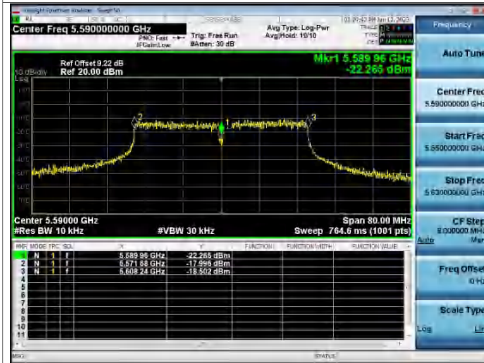
Freq. Stability 0C 120V ac40 5590MHz Ant1 0 Minutes
