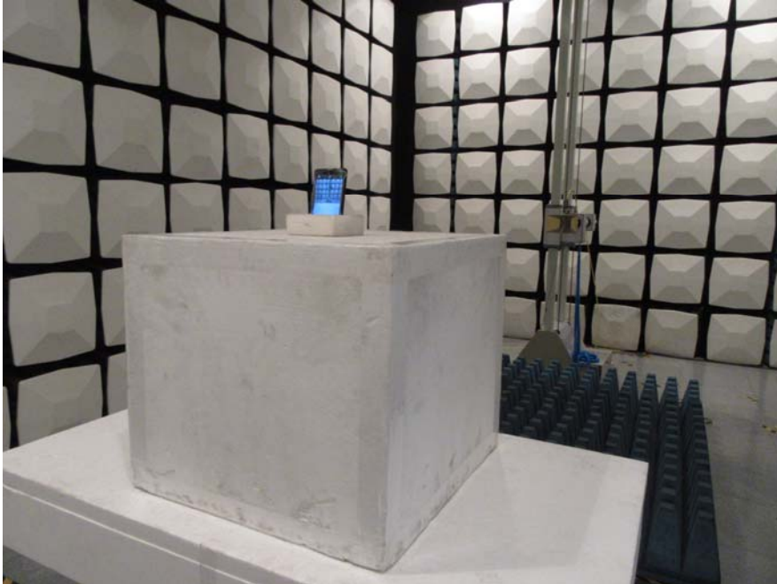
Radiated Emission View (Above 1GHz)
