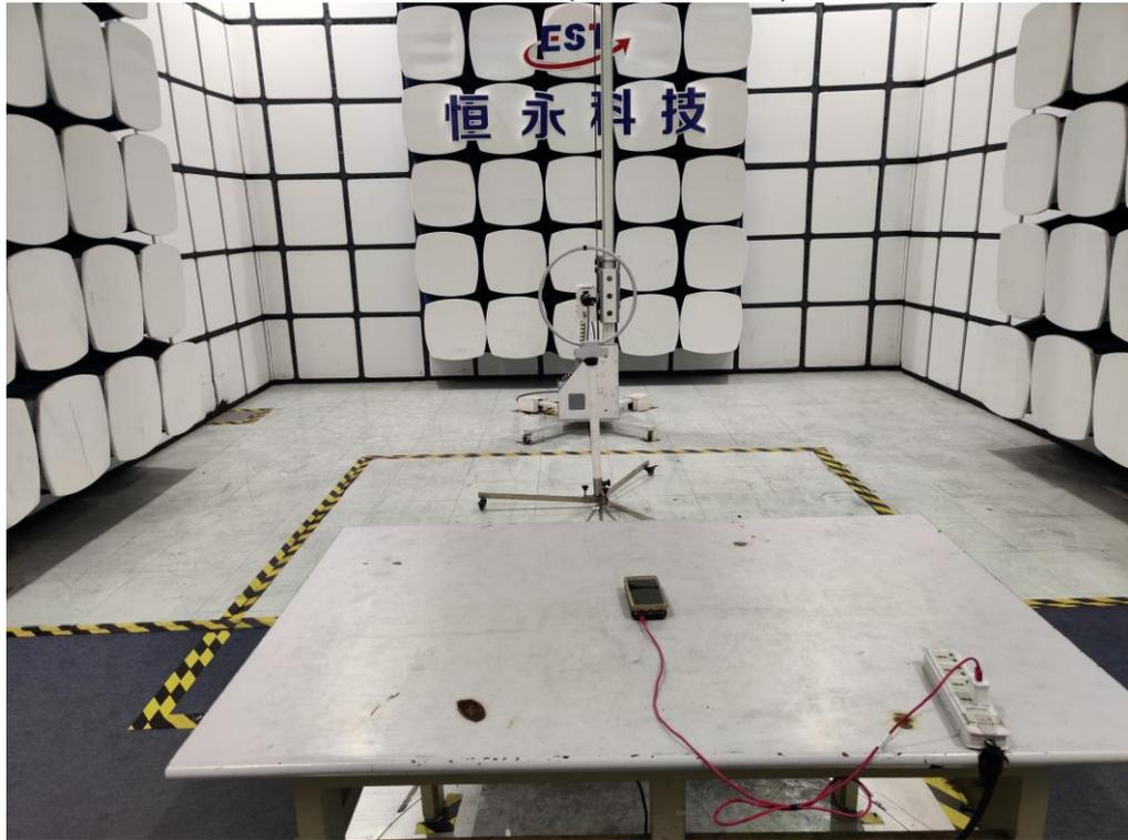
**Radiated Test (30MHz-1GH)**
